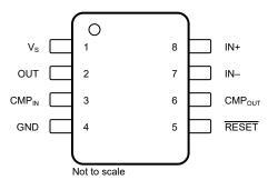
Figure 5-1. INA310x-Q1: DGK Package 8-Pin VSSOP Top View
