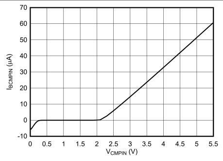
Figure 7-3. Comparator I<sub>BCMPIN</sub> vs V<sub>CMPIN</sub>
