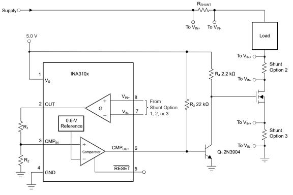
Figure 8-3. Low-Side Switch Overcurrent Shutdown
