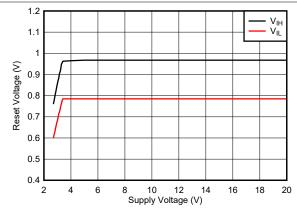
Figure 6-38. Comparator Reset Voltage vs Supply Voltage
