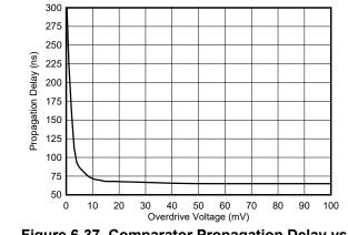
Figure 6-37. Comparator Propagation Delay vs Overdrive Voltage
