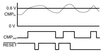
Figure 7-2. The Comparator RESET Function
