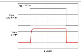
Figure 6-40. Comparator Propagation Delay
