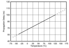
Figure 6-39. Comparator Propagation Delay vs
