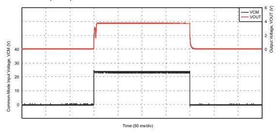
Figure 8-2. Solenoid Control Current Response
