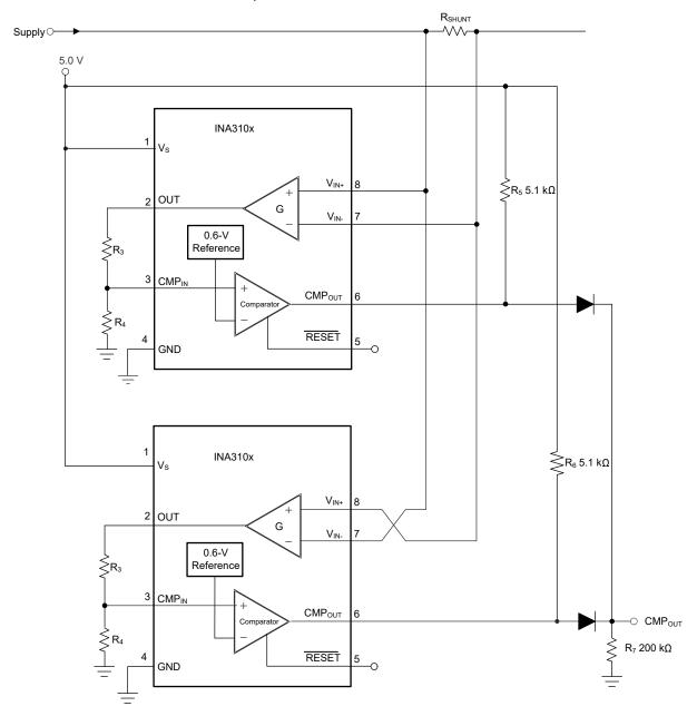
Figure 7-6. Ground Referenced Output
