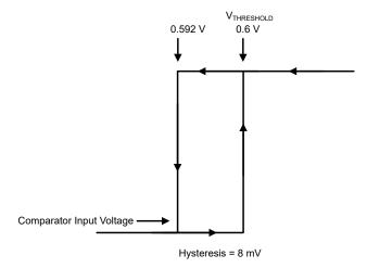
Figure 7-1. The Comparator Threshold and Hysteresis
