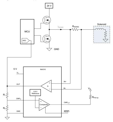
Figure 8-1. Current Sensing in a Solenoid Application
