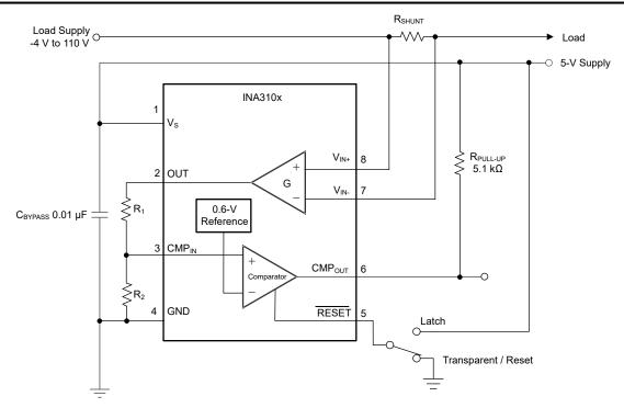
Figure 7-4. INA310x-Q1 Basic Connections
