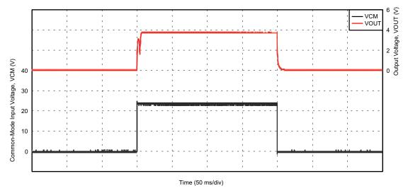
Figure 8-2. Solenoid Control Current Response
