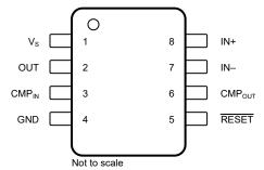
Figure 5-1. INA310x-Q1: DGK Package 8-Pin VSSOP Top View
