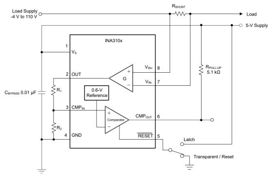
Figure 7-4. INA310x-Q1 Basic Connections
