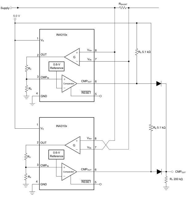
Figure 7-6. Ground Referenced Output
