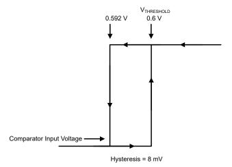
Figure 7-1. The Comparator Threshold and Hysteresis
