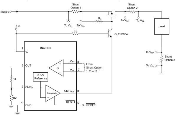
Figure 7-5. High-Side Switch for Overcurrent Shutdown
