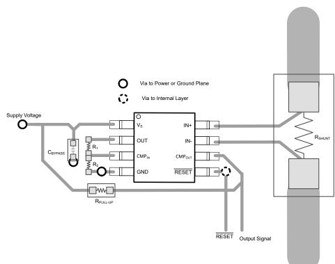
Figure 8-5. INA310x-Q1 Recommended Layout
