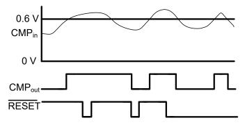
Figure 7-2. The Comparator RESET Function
