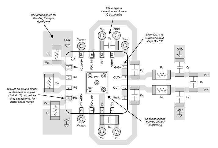
Figure 9-14. Example Schematic and Associated PCB Layout
