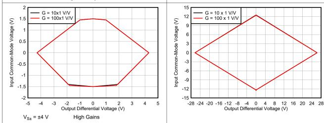
Figure 8-7. Input Common-Mode Voltage vs Output | Figure 8-8. Input Common-Mode Voltage vs Output Voltage, High Gains
