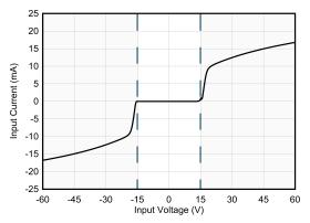
Figure 8-10. Input Current During an Overvoltage Condition
