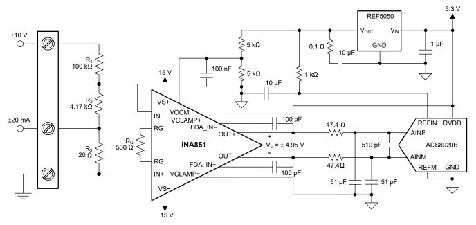
Figure 9-3. PLC Input with INA851 (±10 V, 4 mA to 20 mA)
