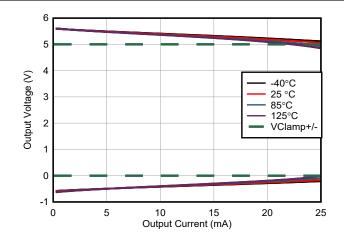
Figure 8-13. Output Voltage With Output Clamping Enabled
