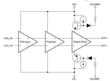
Figure 8-12. Simplified Schematic of Output Driver Clamping Structure
