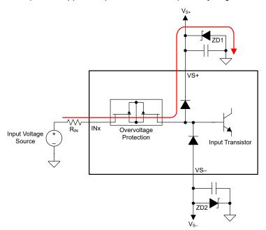
Figure 8-11. Input Current Path During an Overvoltage Condition
