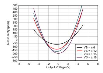
Figure 9-2. Linearity vs Supply Voltage for G = 1000
