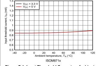
Figure 7-1. Input Threshold Current vs Ambient Temperature
