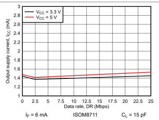
Figure 7-14. Output Supply Current vs Data Rate
