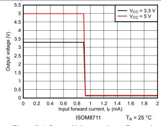
Figure 7-4. Output Voltage vs Input Forward Current
