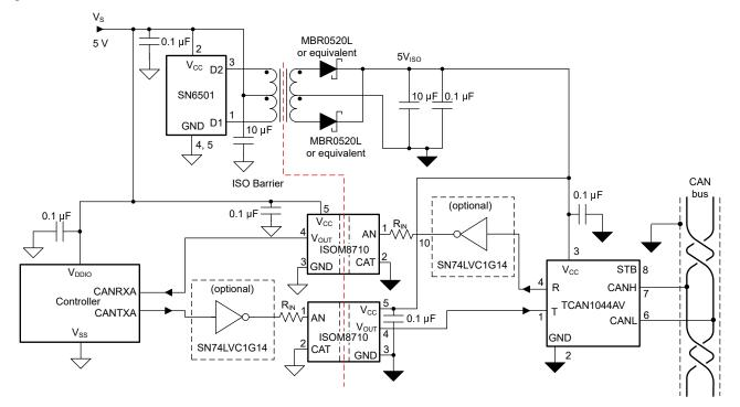
Figure 10-1. Typical Isolated CAN Application Using ISOM8710
