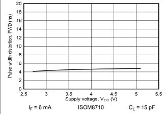
Figure 7-25. Pulse Width Distortion vs Supply Voltage
