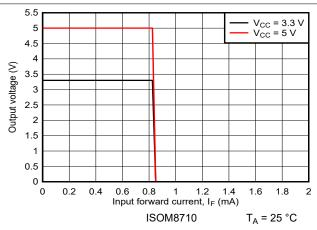
Figure 7-3. Output Voltage vs Input Forward Current
