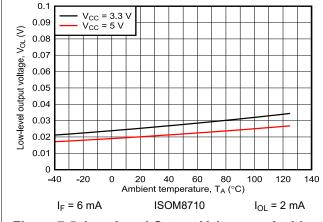
Figure 7-5. Low-Level Output Voltage vs Ambient Temperature
