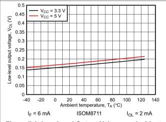
Figure 7-6. Low-Level Output Voltage vs Ambient Temperature
