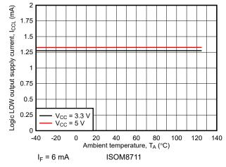
Figure 7-15. Logic LOW Output Supply Current vs
