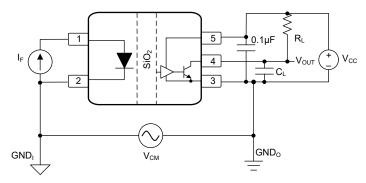
Figure 8-6. ISOM8711 Test Circuit for Common-Mode Transient Immunity
