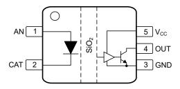
Figure 6-2. ISOM8711 DFF Package, 5-Pin SOIC (Top View)
