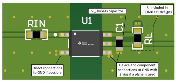
Figure 10-8. Layout Example of ISOM871x with a 2-Layer Board
