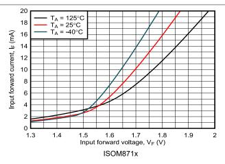
Figure 7-2. Input Forward Current vs Input Forward Voltage
