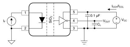
Figure 8-2. ISOM8710 Current-Source Test Circuit for  $I_{CCL}$ ,  $I_{CCH}$ , and Switching Timing
