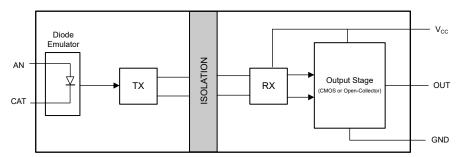
Figure 9-1. Conceptual Block Diagram of an Opto-emulator
