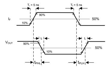
Figure 8-4. Switching Timing Waveforms
