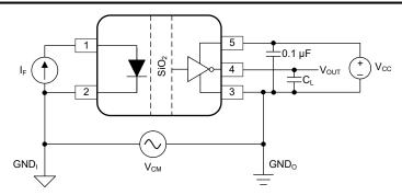
Figure 8-5. ISOM8710 Test Circuit for Common-Mode Transient Immunity
