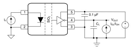
Figure 8-1. ISOM8710 Current-Source Test Circuit for V<sub>OL</sub> and V<sub>OH</sub>
