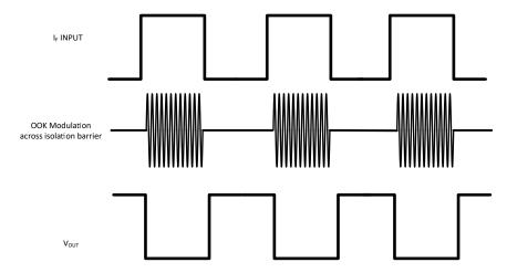
Figure 9-2. On-off Keying (OOK) Based Modulation Scheme
