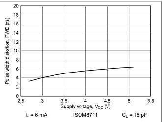
Figure 7-26. Pulse Width Distortion vs Supply Voltage
