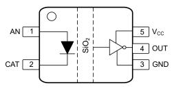
Figure 6-1. ISOM8710 DFF Package, 5-Pin SOIC (Top View)
