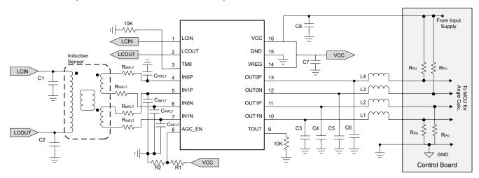
Figure 7-3. Application Schematic - 3.3-V Supply Mode
