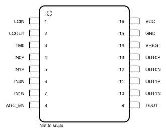
Figure 4-1. PW Package 16-Pin TSSOP Top View
