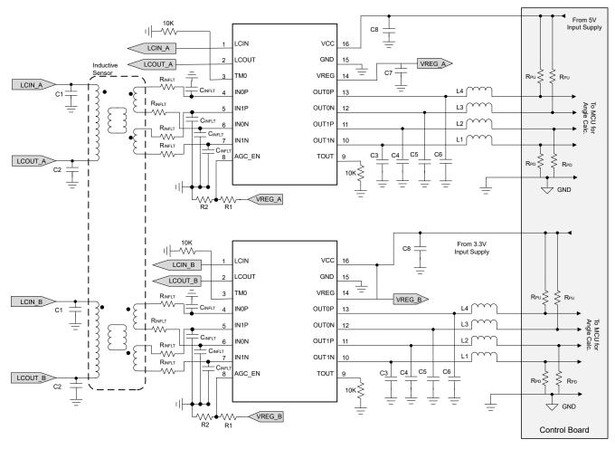
Figure 7-4. Application Schematic - Redundancy Mode
