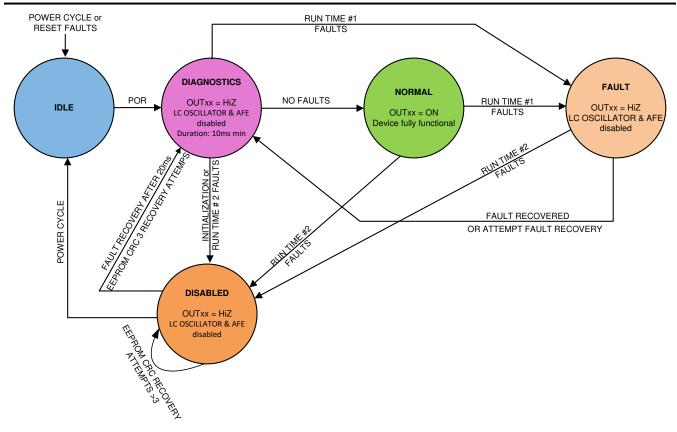
Figure 6-5. Device State Diagram
