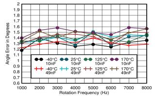
$\rm VCC=3.3V,\, LC_{freq}\text{=}5MHz,\, Ideal\, Inputs,\, No\, offset\, and\, gain\, correction\, Signal\, path\, delay\, compensated$
