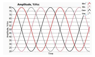
Figure 6-1. LDC5071-Q1 Typical Output
