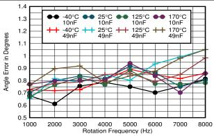
VCC = 3.3V,  $LC_{freq}=5MHz$ , Ideal Inputs, With offset and gain correction Signal path delay compensated
