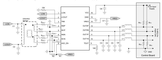
Figure 7-1. Application Schematic - 5-V Supply Mode
