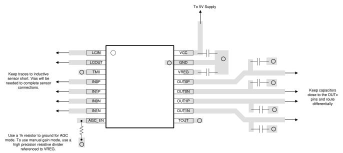
Figure 7-6. Layout Recommendation for the LDC5071-Q1
