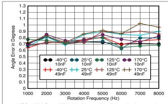
VCC = 5V,  $\rm LC_{freq} = 5MHz, \, Ideal \, Inputs, \, No \, offset \, and \, gain \, correction \, Signal \, path \, delay \, compensated$
