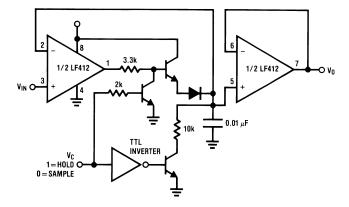
Figure 29. Single Supply Sample and Hold
