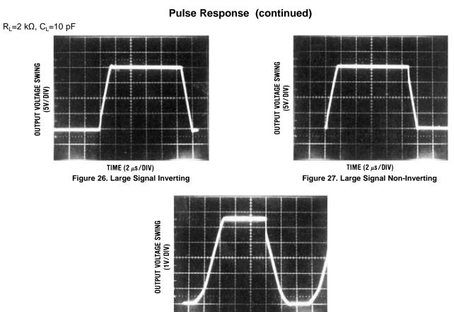
TIME (5  $\mu$ s/DIV) Figure 28. Current Limit (R<sub>L</sub>=100 $\Omega$ )
