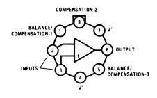
Figure 2. TO-99 Top View See Package Number LMC
