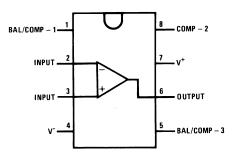
Figure 3. CDIP Package Top View See Package Number NAB0008A
