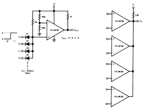
Figure 16. Large Fan-In AND Gate
