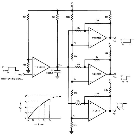
Figure 18. Time Delay Generator
