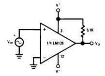
Figure 31. Zero Crossing Detector
