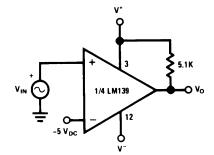
Figure 32. Comparator With a Negative Reference
