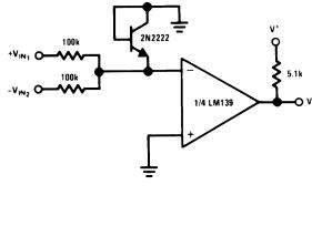
Figure 24. Comparing Input Voltages of Opposite Polarity
