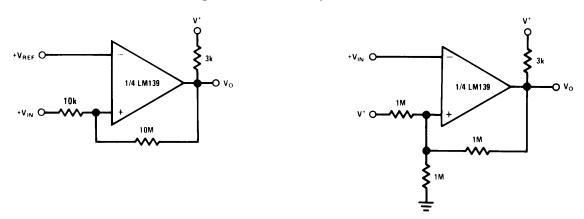
Figure 19. Non-Inverting Comparator with Hysteresis
