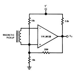
Figure 27. Transducer Amplifier
