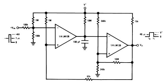
Figure 14. One-Shot Multivibrator with Input Lock Out
