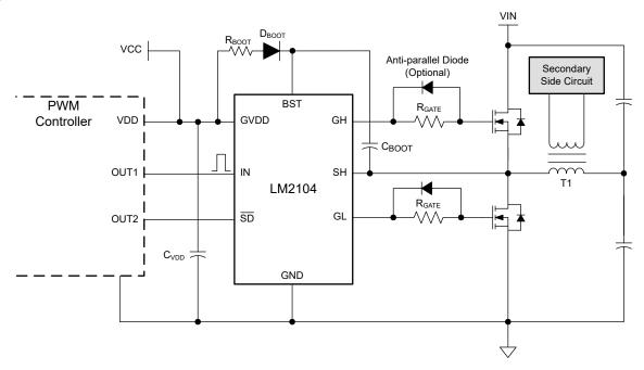
Figure 8-1. LM2104 Driving MOSFETs in a Half-Bridge Converter
