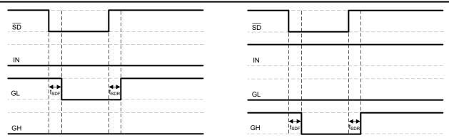
Figure 6-2. Shutdown Timing Diagram
