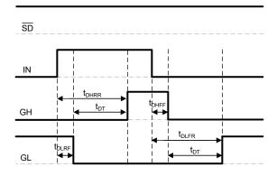
Figure 6-1. Timing Definition Diagram
