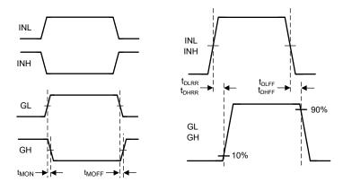
**Figure 6-1. Timing Definition Diagram**
