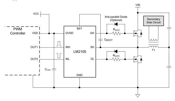
Figure 8-1. LM2105 Driving MOSFETs in a Half-Bridge Converter
