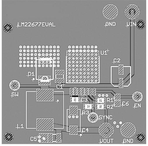
Figure 23. PCB Layout Example
