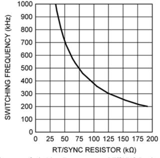
Figure 12. Switching Frequency vs RT/SYNC Resistor
