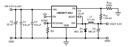
Figure 19. Typical Buck Regulator Application
