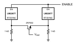
Figure 13. Self Synchronizing Setup
