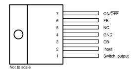
Figure 5-2. NDZ Package 7-Pin TO-220 Top View
