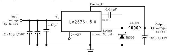
Figure 8-1. Basic Circuit for All Output Voltage Versions
