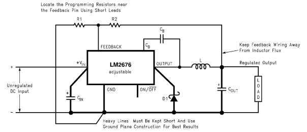
Figure 8-7. Basic Circuit for Adjustable Output Voltage Applications
