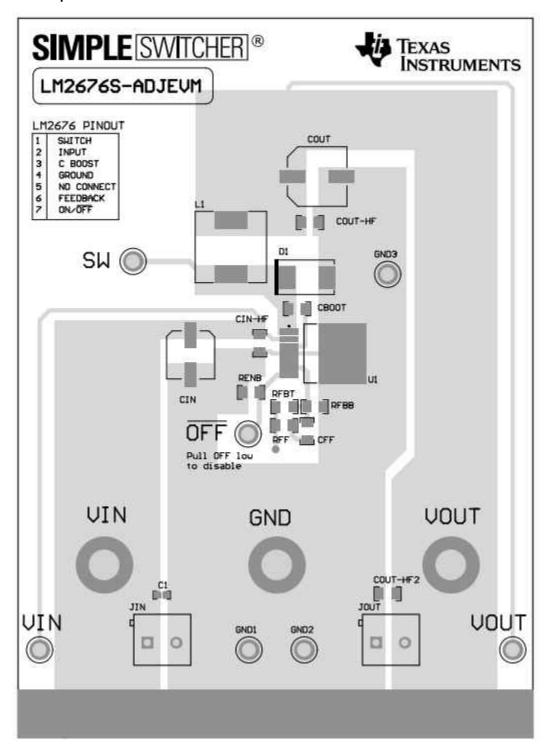
Figure 8-9. LM2676 Layout Example
