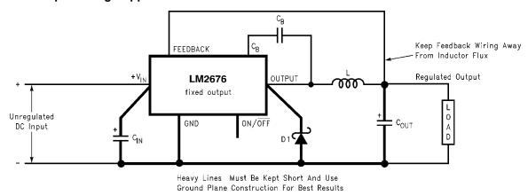
Figure 8-6. Basic Circuit for Fixed Output Voltage Applications.
