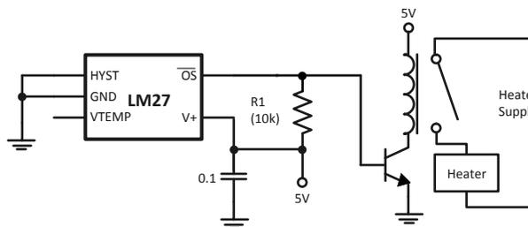
Figure 11. Simple Thermostat
