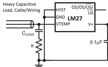
**Figure 5. R in series with capacitor**
