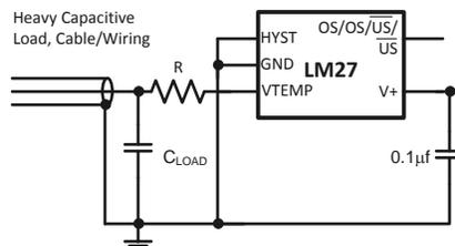
**Figure 6. R in series with signal path**
