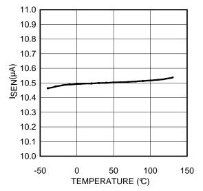
Figure 11. I<sub>SEN</sub> vs Temperature
