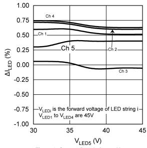
Figure 8. Current Regulation vs V<sub>LED</sub>
