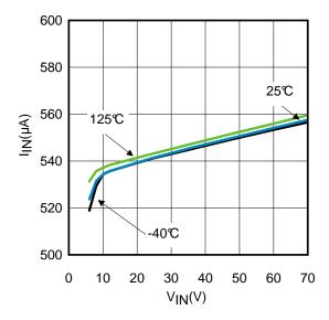
Figure 3. Quiescent Current,  $I_{\text{IN}}$  vs  $V_{\text{IN}}$
