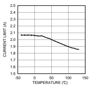
Figure 12. Current Limit vs Temperature
