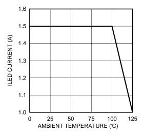
Figure 18. Thermal Derating Curve for the eDDA-8 Package
