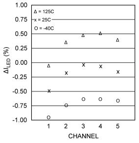
Figure 5. Current Regulation (Channel to Channel) vs Temperature
