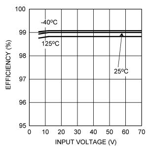
Figure 6. Efficiency vs V<sub>IN</sub>
