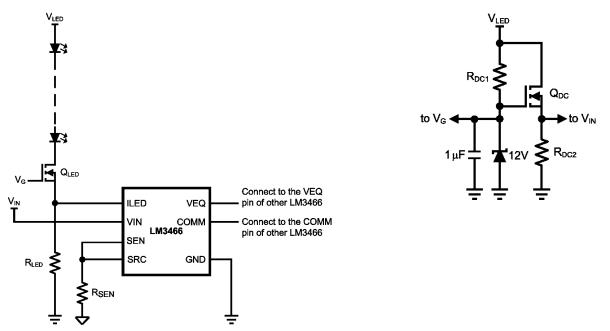
Figure 16. External MOSFET Circuit for High **Voltage Applications**
