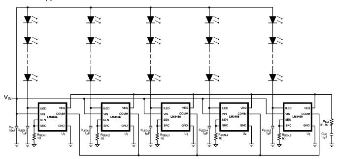
Figure 19. Application Circuit of a LM3466 Lighting System
