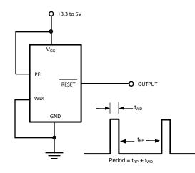
Figure 18. LM3710 Long Period oscillator
