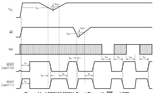
Figure 11. LM3710/LM3711 Reset Time with MR and WDI
