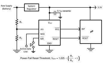
Note:  $\overline{MR}$  input with its 1.225V nominal threshold, may monitor an additional supply voltage. An internal 56 k $\Omega$  pull-up resistor is included on this input.
