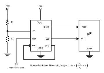
Figure 14. Monitoring Two Critical Supplies And Dataline
