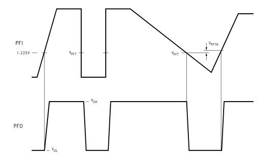
Figure 13. PFI Comparator Timing Diagram
