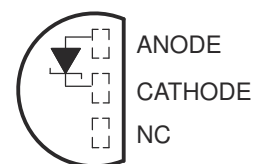
1.2 V . . . LP (TO-92/TO-226) PACKAGE (TOP VIEW)
