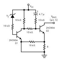
Figure 46. External Undervoltage Pull-Down
