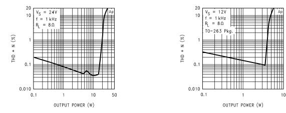
Figure 45. THD+N vs. P<sub>OUT</sub> for Bridge-Mode Application
