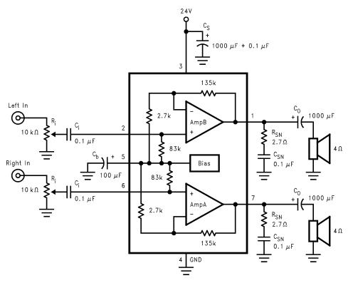
Figure 5. Circuit for External Components Description
