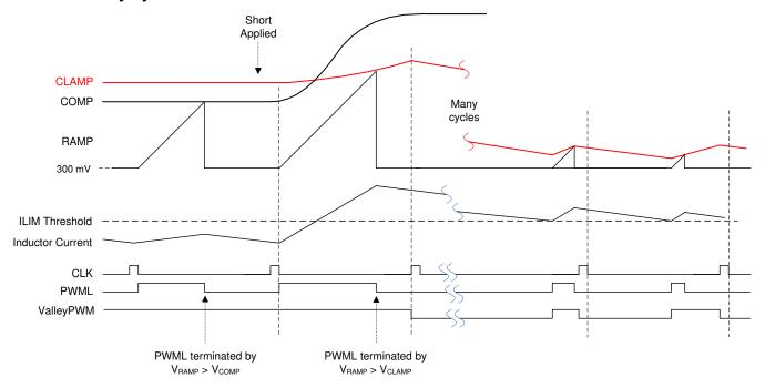
Figure 8-11. OCP Duty Cycle Limiting Waveforms
