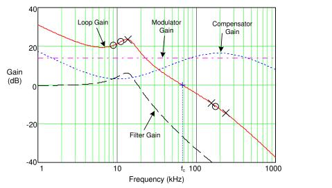
Figure 9-3. Buck Regulator Constituent Gain Components
