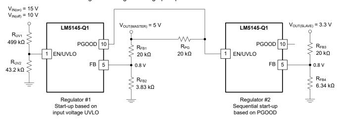
Figure 8-4. Master-Slave Sequencing Implementation Using PGOOD and EN/UVLO
