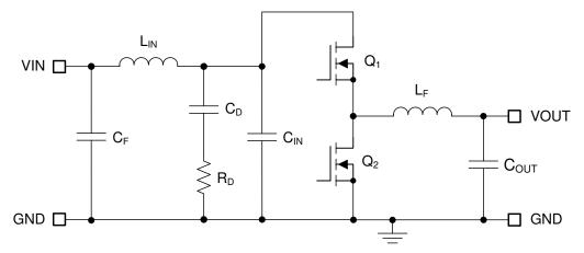
Figure 9-4. Buck Regulator With π-Stage EMI Filter
