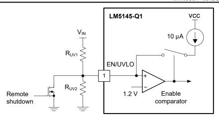
Figure 8-3. Programmable Input Voltage UVLO Turn-on and Turn-off
