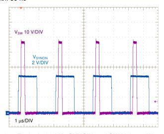
Figure 8-5. Typical 400-kHz SYNCIN and SW Voltage Waveforms
