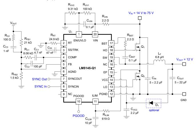
Figure 9-16. Application Circuit 2 With LM5145-Q1 48-V to 12-A Synchronous Buck Regulator at 400 kHz
