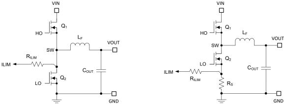
Figure 8-8. MOSFET R<sub>DS(on)</sub> Current Sensing
