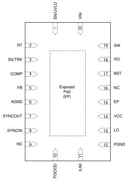
Connect Exposed Pad on bottom to AGND and PGND on the PCB.
