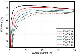
Typical Application Circuit and Efficiency Performance,  $V_{OUT}$  = 12 V,  $F_{SW}$  = 400 kHz
