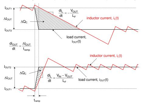
Figure 9-1. Load Transient Response Representation Showing Cour Charge Surplus or Deficit
