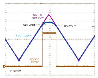
Figure 8-6. Typical Output Voltage Tracking and PGOOD Waveforms
