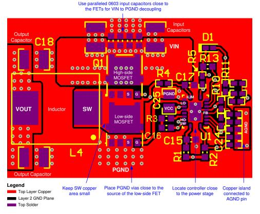
Figure 11-2. LM5145-Q1 Controller PCB Layout (Viewed From Top)
