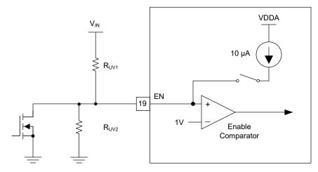
Figure 8-2. Programmable Input Voltage UVLO Turn-On
