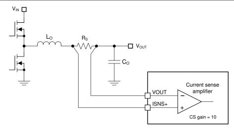
Figure 8-4. Shunt Current Sensing Implementation
