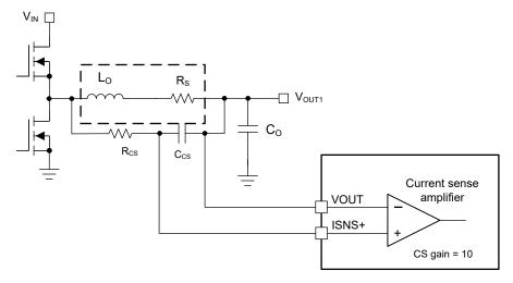
Figure 8-5. Inductor DCR Current Sensing Implementation
