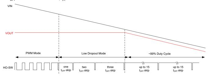
Figure 8-1. Dropout Mode Operation
