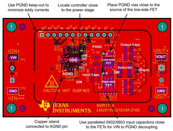
Figure 9-47. PCB Top Layer – High Density, Single-sided Design
