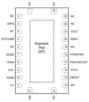
Connect the exposed pad to AGND and PGND on the PCB.
