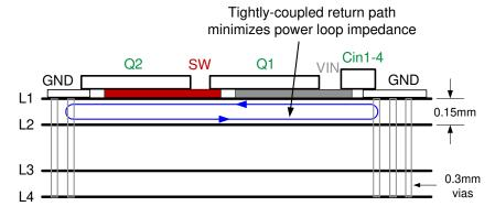
Figure 9-49. PCB Stack-up Diagram With Low L1-L2 Intra-layer Spacing <sup>1</sup>
