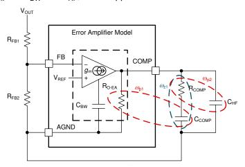
Figure 9-3. Error Amplifier and Compensation Network
