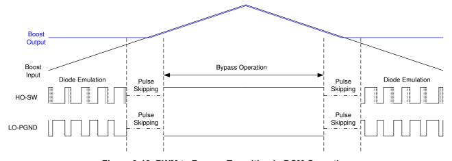
Figure 9-19. PWM to Bypass Transition in DCM Operation
