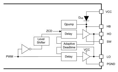
Figure 9-20. Driver Structure with Internal Boot Diode
