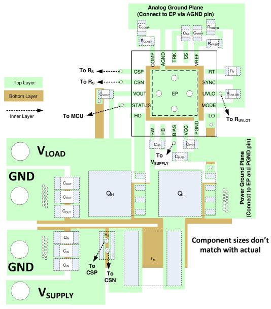
Figure 12-1. PCB Layout Example
