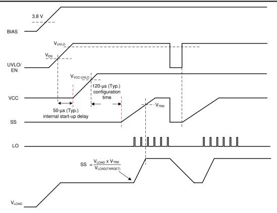
Figure 9-5. Boost Start-Up Waveforms Case 2: Start-Up by EN/UVLO, Restart when VH > V<sub>SYNC</sub>
