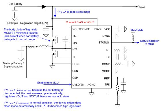
Figure 10-8. LM51521 in Emergency Call/Backup Battery Booster Application
