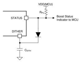
Figure 10-3. Enable Both Clock Dithering and Bypass Operation
