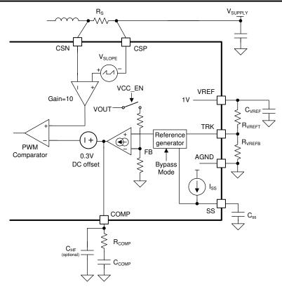
Figure 9-14. Error Amplifier, Current Sense Amplifier, and PWM
