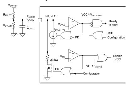
Figure 9-1. EN/UVLO Circuit
