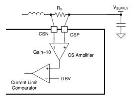
Figure 9-16. Current Limit Comparator
