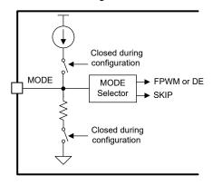
Figure 9-3. MODE Selection Circuit
