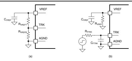
Figure 9-6. TRK Control (a) Using VREF (b) by External Step Input
