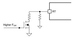
Figure 9-8. Frequency Hopping Example
