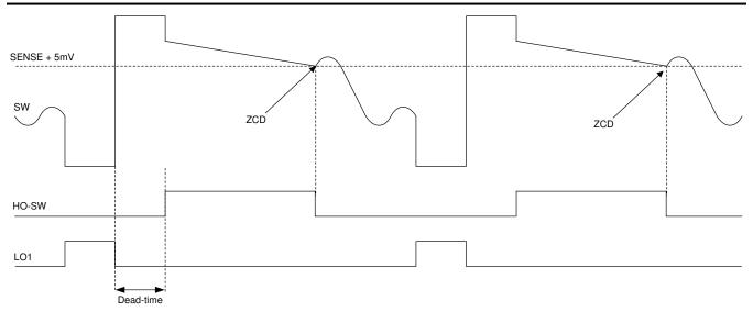
Figure 9-23. Zero Current Detection
