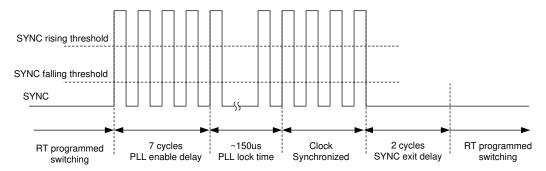
Figure 9-9. External Clock Synchronization
