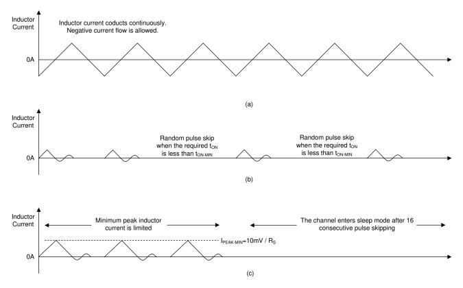
Figure 9-22. Inductor Current Waveform at Light Load (a) FPWM (b) Diode Emulation (c) Skip Mode
