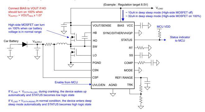
Figure 10-7. LM5152-Q1 in Automotive Pre-boost Application
