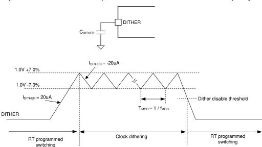
Figure 9-10. Switching Frequency Dithering
