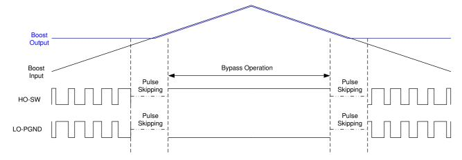
Figure 9-18. PWM to Bypass Transition in CCM Operation
