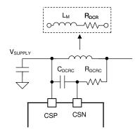
Figure 10-2. DCR Current Sensing
