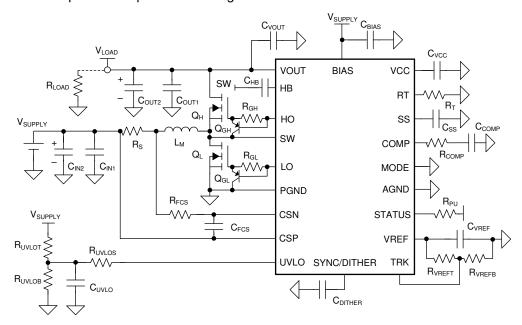
Figure 10-1. Typical Synchronous Boost Converter with Optional Components
