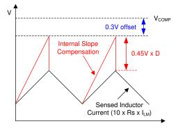
Figure 9-15. PWM Comparator Input
