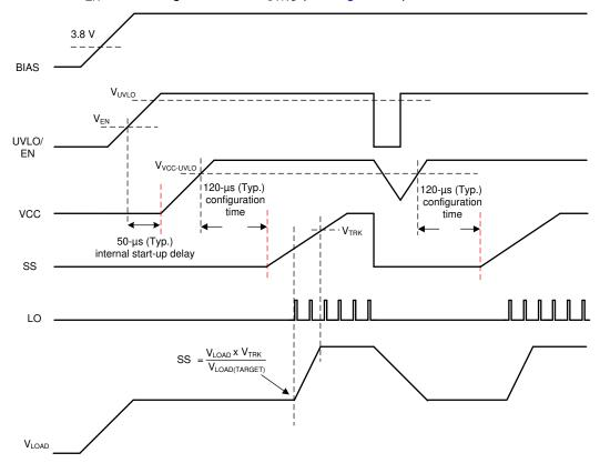
Figure 9-4. Boost Start-Up Waveforms Case 1: Start-Up by EN/UVLO, Restart when VH < V<sub>SYNC</sub>
