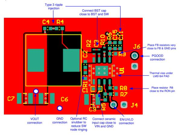
Figure 7-19. LM5164 Single-Sided PCB Layout Example
