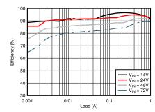
Typical Application Efficiency, V<sub>OUT</sub> = 12V
