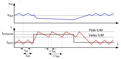
Figure 6-1. Current Limit Timing Diagram
