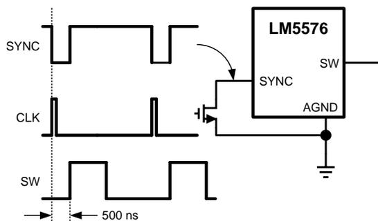
Figure 11. Sync from External Clock
