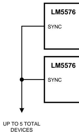
Figure 12. Sync from Multiple Devices
