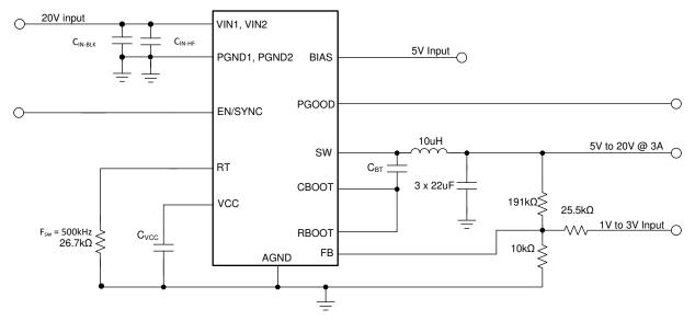
Figure 9-44. USB Type-C Power Supply
