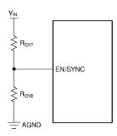
Figure 9-4. UVLO Using EN
