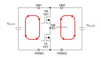
Figure 11-1. Input Current Loop
