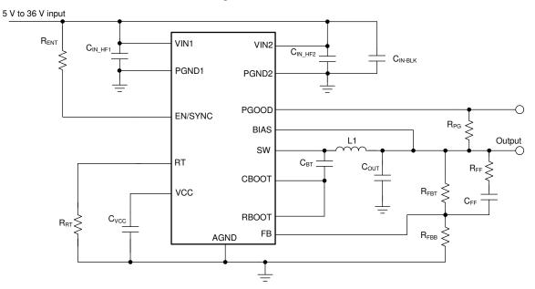
Figure 9-1. Example Application Circuit
