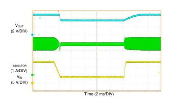
Figure 8-9. Recovery From Dropout
