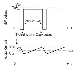
Figure 8-12. Current Limit Waveforms
