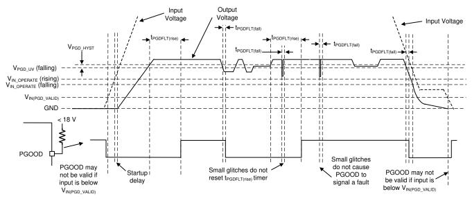
Figure 8-6. PGOOD Timing Diagram (Excludes OV Events)
