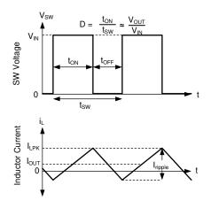
In FPWM mode, Continuous Conduction (CCM) is possible even if I<sub>OUT</sub> is less than half of I<sub>ripple</sub>.
