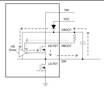
Figure 8-7. Simplified Circuit Showing How RBOOT Functions
