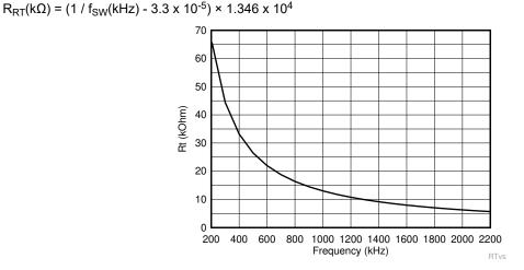
Figure 8-5. Setting Clock Frequency
