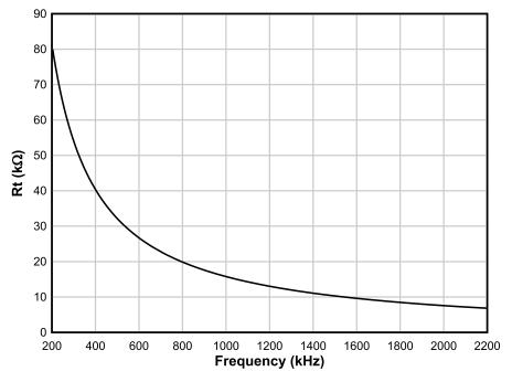
Figure 8-6. Setting Clock Frequency
