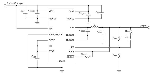
Figure 9-1. Example Application Circuit - 400-kHz Adjustable Output
