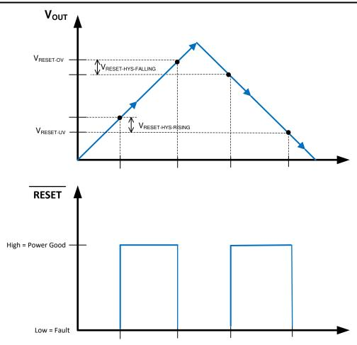
Figure 8-7. RESET Static Voltage Thresholds
