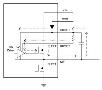
Figure 8-10. Simplified Circuit Showing How RBOOT Functions
