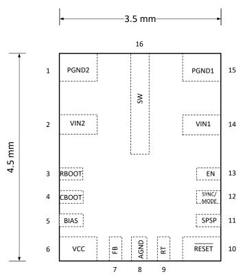
Figure 6-1. 16-Pin VQFN RPH Package (Top View)
