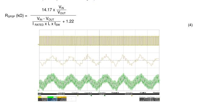
Figure 8-11. Output Ripple Without Ripple Cancellation Showing V<sub>SW</sub> (top), F<sub>SW</sub> (middle), V<sub>OUT</sub> (bottom)
