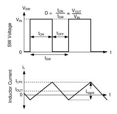
FPWM mode Continuous Conduction (CCM) is possible even if I<sub>OUT</sub> is less than half of Iripple.
