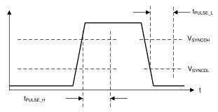
This image shows the conditions needed for detection of a synchronization signal.
