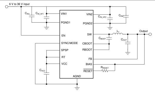
Figure 9-2. Example Application Circuit - 400-kHz Fixed Output
