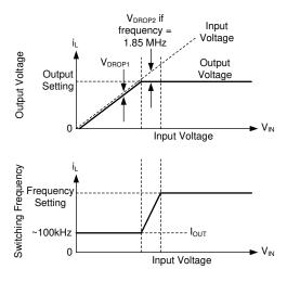
Output voltage and frequency versus input voltage: If there is little difference between input voltage and output voltage setting, the IC reduces frequency to maintain regulation. If input voltage is too low to provide the desired output voltage at approximately 110 kHz, output voltage tracks input voltage.
