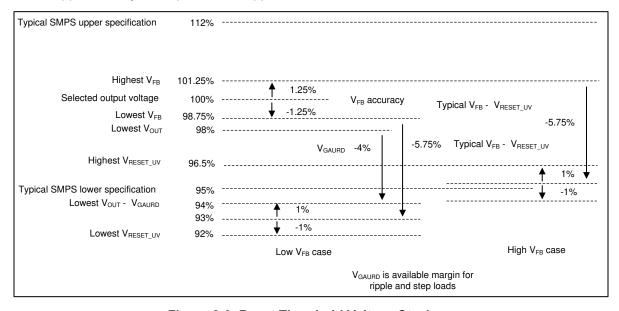
Figure 8-9. Reset Threshold Voltage Stack-up
