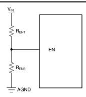
Figure 8-2. VIN UVLO Using the EN Pin
