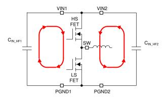
Figure 11-1. Input Current Loop
