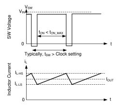
Figure 8-16. Current Limit Waveforms
