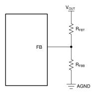
Figure 8-1. Setting Output Voltage of Adjustable Versions
