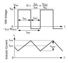
Figure 8-20. SW Voltage and Inductor Current Waveforms in Continuous Conduction Mode (CCM)
