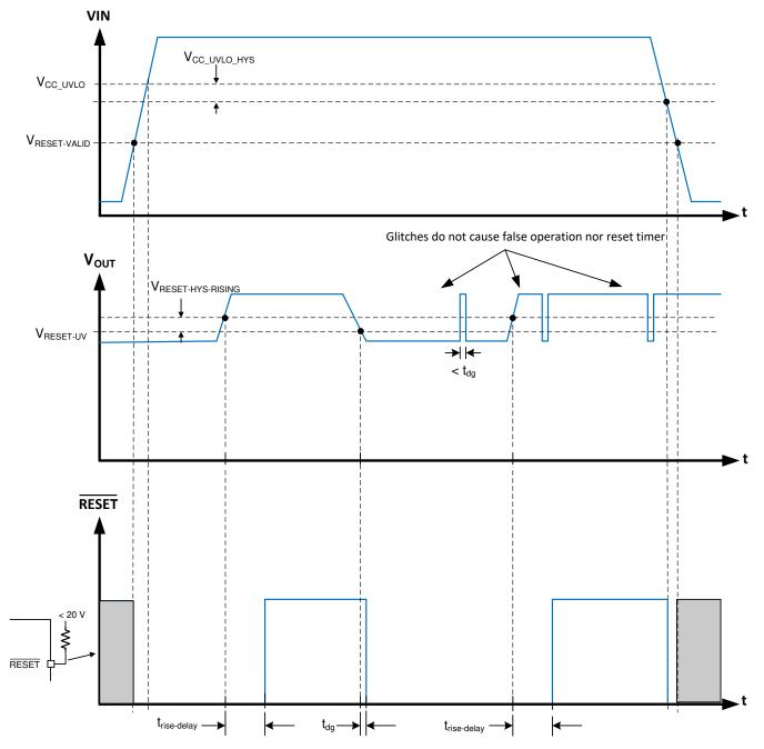
Figure 8-8. RESET Timing Diagram (Excludes OV Events)
