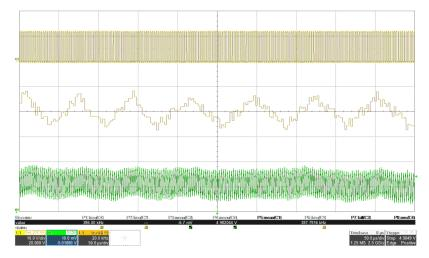
Figure 8-12. Output Ripple with Ripple Cancellation Showing V<sub>SW</sub> (top), F<sub>SW</sub> (middle), V<sub>OUT</sub> (bottom)
