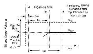
The left curves show soft start from 0 V. The right curves show soft starting behavior from a pre-biased or non-zero voltage. In either case, the output voltage reaches within 10% of the desired setpoint  $t_{SS}$  time after soft start is initiated. During soft start, FPWM and hiccup are disabled. Both hiccup and FPWM are enabled once output reaches regulation or  $t_{SS2}$ , whichever happens first.
