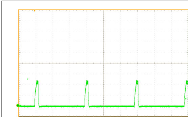
Figure 8-18. Inductor Current Bursts During Hiccup
