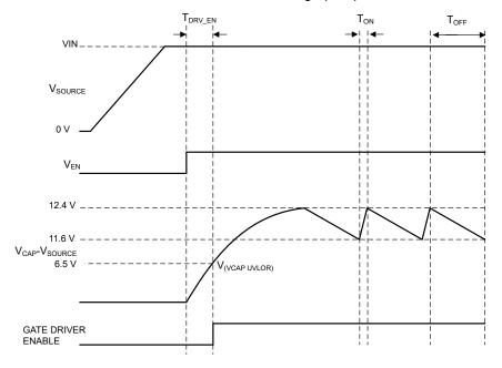
Figure 8-1. Charge Pump Operation
