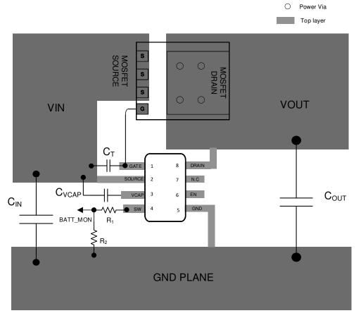
Figure 11-1. LM74501-Q1 Layout Example
