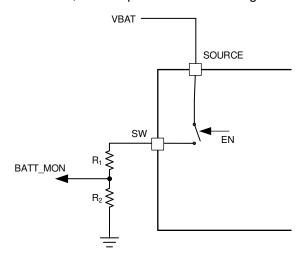
Figure 8-2. LM74501-Q1 SW Functionality
