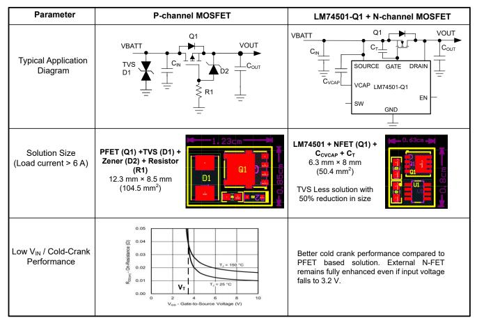
Figure 9-1. PFET vs LM74501-Q1 Reverse Polarity Protection Solution Comparison
