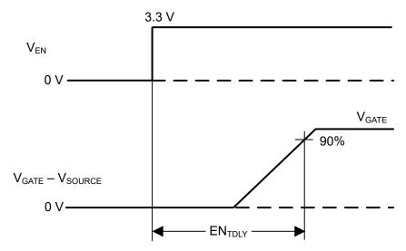
Figure 7-1. Timing Waveforms
