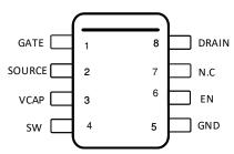
Figure 5-1. DDF Package 8-Pin SOT-23 (LM74501-Q1 Top View)
