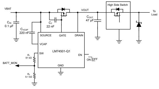
Figure 9-2. Typical Application Circuit
