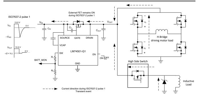
Figure 8-3. Typical Application Scenario During ISO7637-2 Pulse 1 Events
