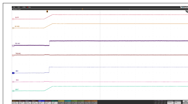
Figure 8-2. +48V DC Input, Startup with Vin Ramp
