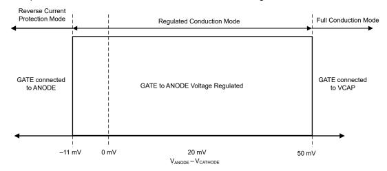
Figure 9-2. Gate Driver Mode Transitions
