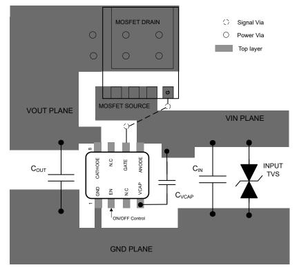
Figure 10-19. LM74700D-Q1 Example Layout
