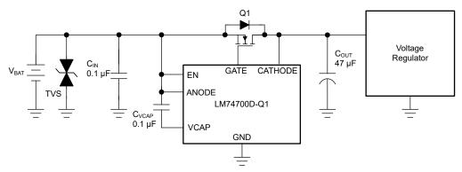
Figure 10-1. Typical Application Circuit
