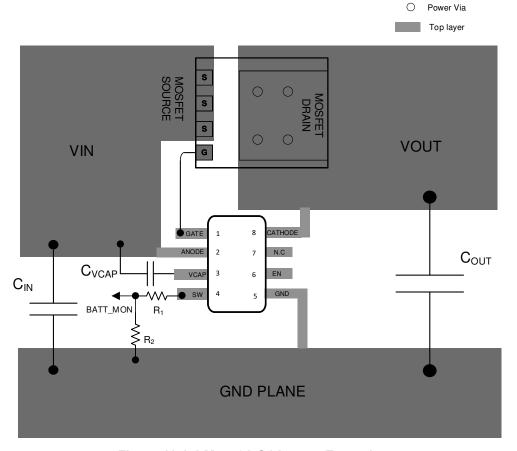
Figure 11-1. LM74701-Q1 Layout Example
