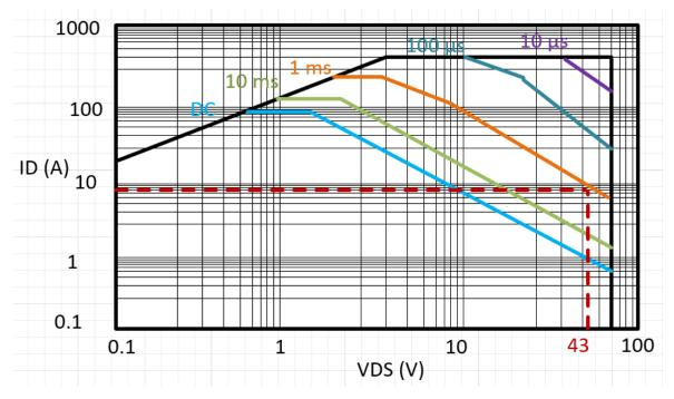
Figure 9-2. Typical MOSFET SoA Characteristics
