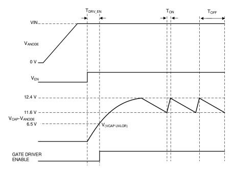
Figure 8-1. Charge Pump Operation
