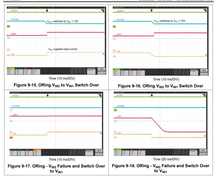
LM74701-Q1 has VDS clamp mode of operation where device detects the voltage difference between CATHODE and ANODE and turns on the external FET in active clamp region when the  $V_{(OUT)} - V_{(IN)}$  crosses the VDS<sub>CLAMP</sub> threshold. So LM74701-Q1 can be used in ORing applications where worst case  $V_{(OUT)} - V_{(IN)}$  is less than device VDS<sub>CLAMP</sub> minimum specification as mentioned in the Electrical Characteristics table.
