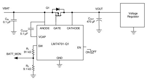
Figure 9-1. Typical Application Circuit
