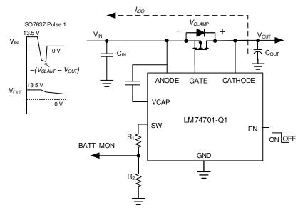
Figure 8-4. LM74701-Q1 Operation During VDS Clamp Mode
