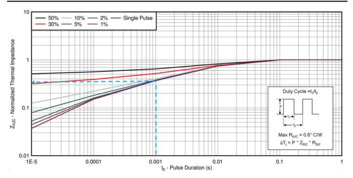
Figure 9-3. Typical MOSFET Transient Thermal Impedance
