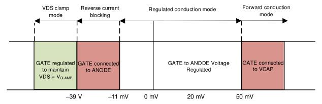
Figure 8-2. Gate Driver Mode Transitions
