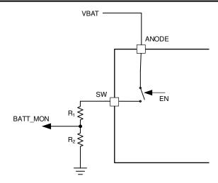
Figure 8-3. LM74701-Q1 SW Pin Functionality
