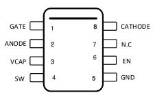
Figure 5-1. DDF Package 8-Pin SOT-23 Top View
