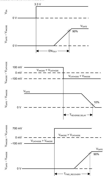
Figure 7-1. Timing Waveforms
