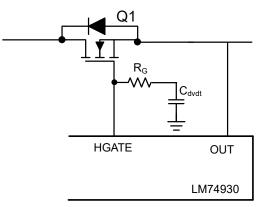
Figure 7-2. Inrush Current Limiting
