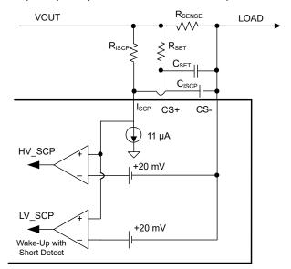
Figure 7-7. Short-Circuit Protection With Deglitch Filter
