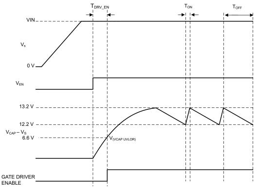
Figure 7-1. Charge Pump Operation
