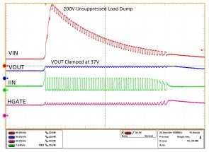
Unsuppressed Load Dump 200 V - Output Clamp
