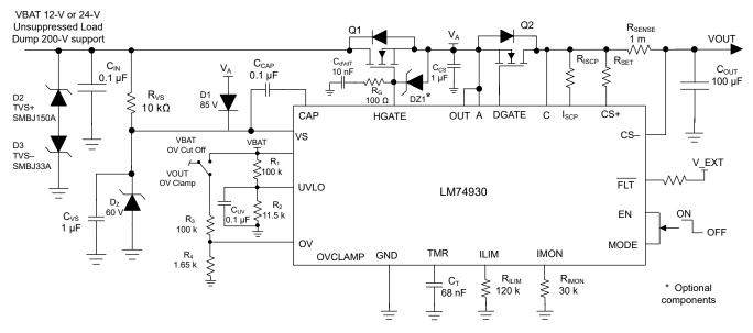
Figure 8-1. Typical Application Circuit: 200-V Unsuppressed Load Dump Protection with Reverse Battery Protection
