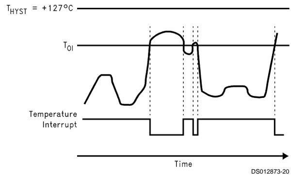
Interrupt resets occur when Interrupt Status Register 1 is read but will set again when monitoring cycle continues (as long as temperature exceeds  $T_{OI}$ ). When temperature descends below  $T_{OI}$  allow up to two monitoring loops before the Temperature Interrupt resets.
