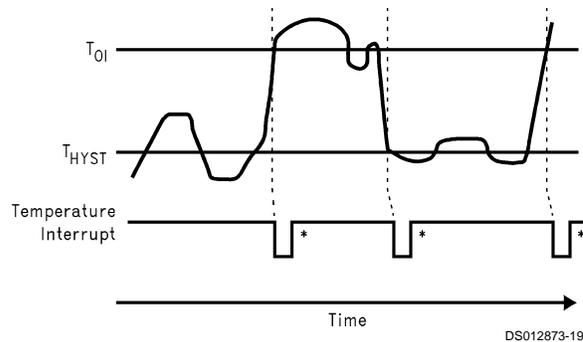
\*Note: Interrupt resets occur only when interrupt Status Register 1 is read.
