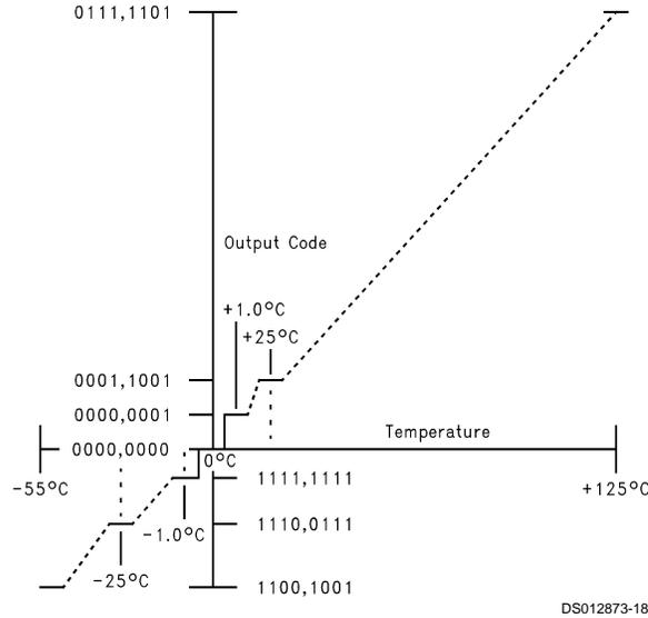
**FIGURE 10. Temperature-to-Digital Transfer Function (Non-Linear Scale for Clarity)**
