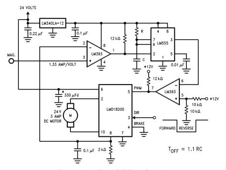
Figure 11-6. Fixed Off-Time Control
