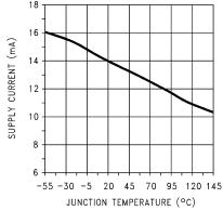
Figure 9-6. Supply Current vs Temperature (V<sub>S</sub> = 42V)
