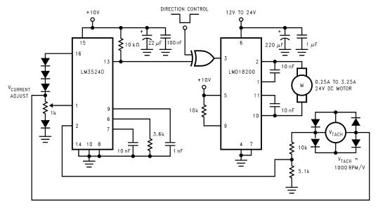
Figure 11-10. Regulate Velocity with Tachometer Feedback
