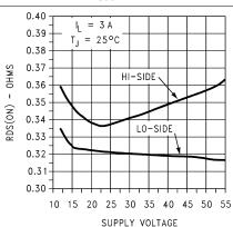
Figure 9-3. R<sub>DS</sub>(On) vs Supply Voltage
