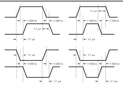
Figure 11-3. Transitions in Brake, Direction, or PWM Must Be Separated By At Least 1 µsec
