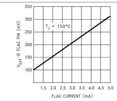
Figure 9-1. V<sub>Sat</sub> vs Flag Current
