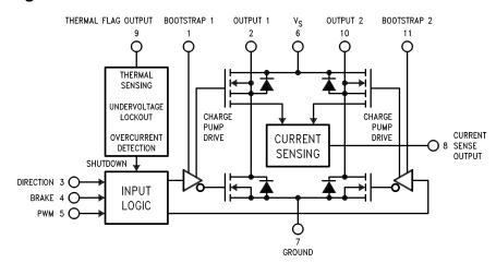
Figure 4-1. Functional Block Diagram of LMD18200
