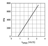
Figure 11-11. Motor Speed vs Control Voltage
