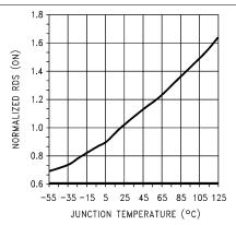
Figure 9-2. R<sub>DS</sub>(On) vs Temperature
