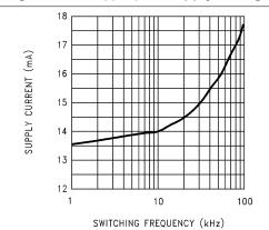
Figure 9-5. Supply Current vs Frequency ( $V_S = 42V$ )
