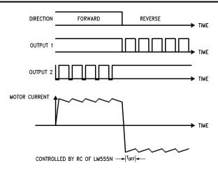
Figure 11-7. Switching Waveforms
