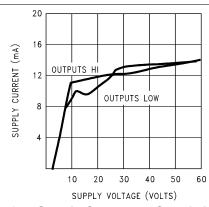
Figure 9-4. Supply Current vs Supply Voltage
