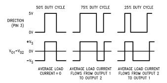
Figure 11-1. Locked Anti-Phase PWM Control
