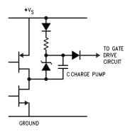
Figure 11-4. Internal Charge Pump Circuitry
