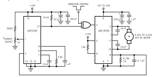
Figure 11-8. Locked Anti-Phase Control Regulates Torque
