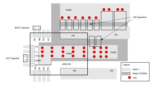
Figure 8-7. External Component Placement (Multi-layer PCB)
