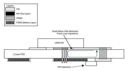
Figure 8-10. Two-Layer Board Cross Section With Return Path
