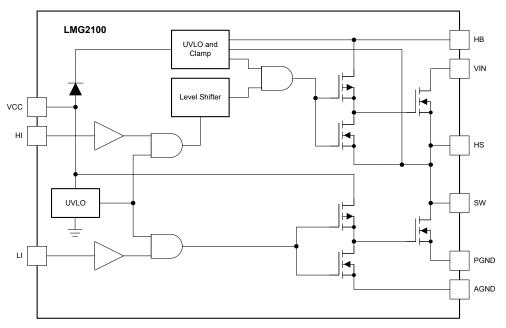
Figure 7-1. Functional Block Diagram
