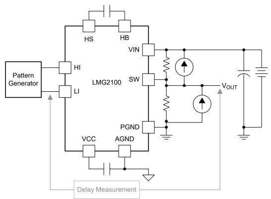
Figure 6-1. Propagation Delay and Propagation Mismatch Measurement
