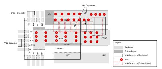
Figure 8-9. External Component Placement (Double Layer PCB)
