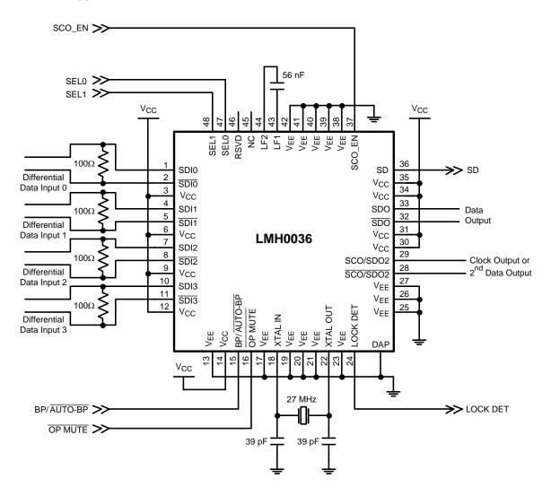
Figure 5. Application Circuit
