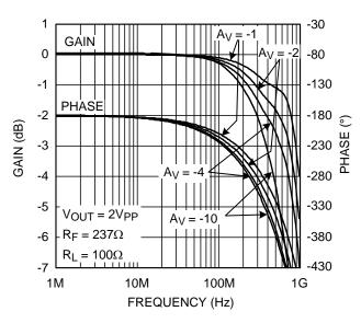
Figure 3. Inverting Frequency Response
