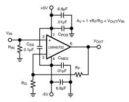
Figure 21. Recommended Non-Inverting Gain Circuit
