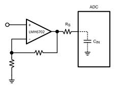
Figure 24. Input Amplifier to ADC
