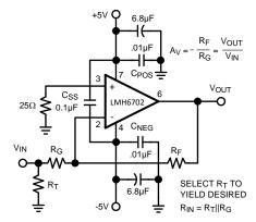
Figure 22. Recommended Inverting Gain Circuit
