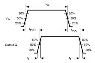
Figure 21. Propagation Delay
