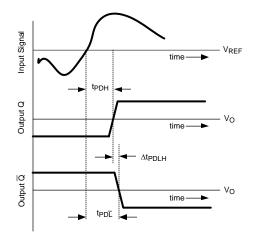
Figure 22. t<sub>PD</sub> with Complementary Outputs
