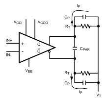
Figure 30. Parasitic Capacities
