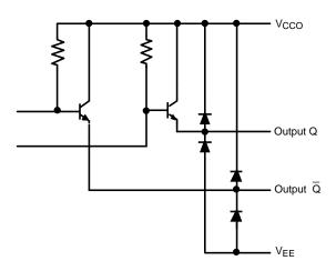
Figure 14. Equivalent Output Circuitry
