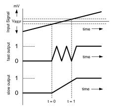
Figure 26. Oscillations on Output Signal
