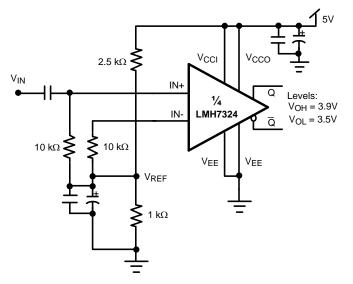
Figure 20. Standard Setup
