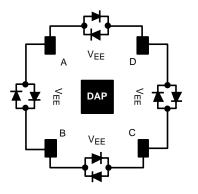
Figure 16. DAP and V<sub>EE</sub> Configuration
