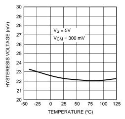
Figure 28. Hysteresis Voltage over Temperature
