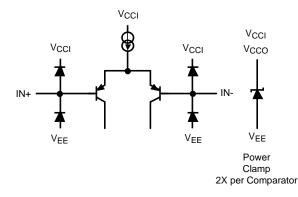
Figure 13. Equivalent Input Circuitry
