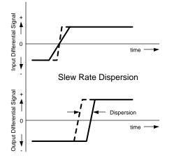
Figure 24. Slew Rate Dispersion
