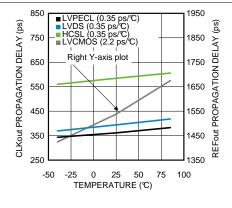
Figure 17. Propagation Delay vs. Temperature
