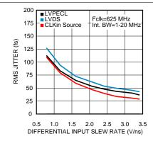
Figure 13. RMS Jitter vs. CLKin Slew Rate at 156.25 MHz
