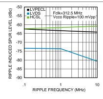
Figure 16. PSRR vs. Ripple Frequency at 312.5 MHz
