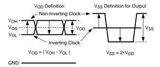
Figure 24. Two Different Definitions for Differential Output Signals
