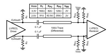
Figure 35. Differential LVPECL Operation, AC Coupling, Thevenin Equivalent
