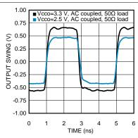
Figure 7. HCSL Output Swing at 250 MHz
