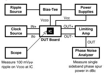
Figure 39. PSRR Test Setup
