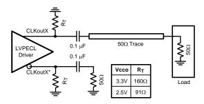
Figure 38. Single-Ended LVPECL Operation, AC Coupling
