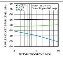
Figure 15. PSRR vs. Ripple Frequency at 156.25 MHz
