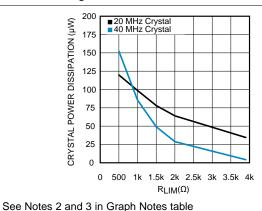
Figure 21. Crystal Power Dissipation vs. R<sub>LIM</sub>
