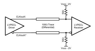
Figure 31. Differential LVPECL Operation, DC Coupling
