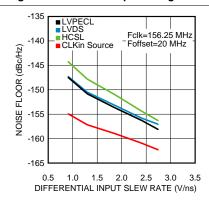
Figure 9. Noise Floor vs. CLKin Slew Rate at 100 MHz
