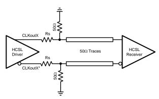
Figure 30. HCSL Operation, DC Coupling
