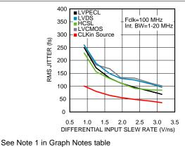
Figure 11. Noise Floor vs. CLKin Slew Rate at 625 MHz
