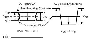
Figure 23. Two Different Definitions for Differential Input Signals
