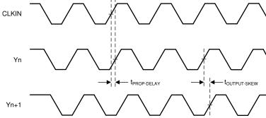
Figure 8-6. Propagation Delay  $t_{\mbox{\scriptsize PROP-DELAY}}$  and Output Skew  $t_{\mbox{\scriptsize OUTPUT-SKEW}}$
