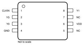
Figure 6-1. LMK1C1102 PW Package 8-Pin TSSOP Top View
