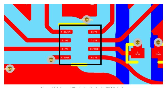
Figure 12-2. Layout illustration for 8-pin WSON device
