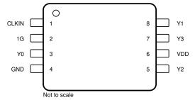
Figure 6-4. LMK1C1104 PW Package 8-Pin TSSOP Top View
