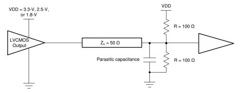
Figure 8-2. Application Load With 50-Ω Termination
