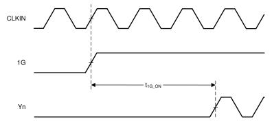
Figure 8-4.  $t_{1G\ ON}$  Output Enable Time
