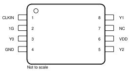
Figure 6-3. LMK1C1103 PW Package 8-Pin TSSOP Top View
