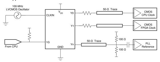
Figure 10-1. System Configuration Example
