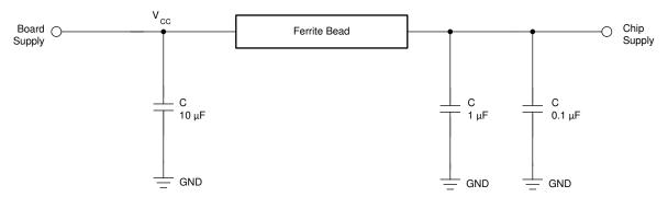
Figure 11-1. Power Supply Decoupling
