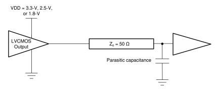
Figure 8-3. Application Load With Termination
