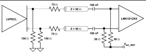
Figure 9-5. LVPECL Clock Driver Connected to LMK1D121x Input
