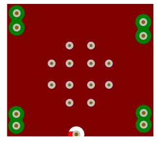
Figure 10-6. PCB Layout Example for LMK1D1212, GND Layer
