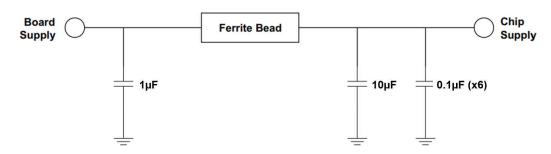
Figure 10-4. Power Supply Decoupling
