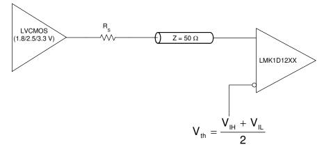
Figure 9-6. 1.8-V, 2.5-V, or 3.3-V LVCMOS Clock Driver Connected to LMK1D121x Input
