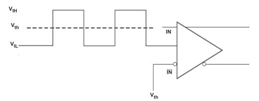
Figure 8-3. DC-Coupled LVCMOS Input During Device Test
