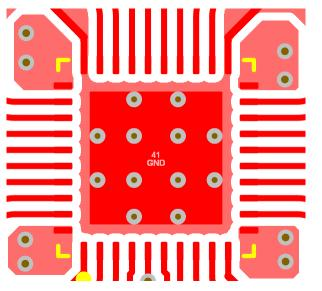
Figure 10-5. PCB layout example for LMK1D1212, Top Layer
