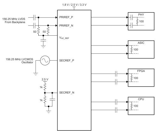
Figure 10-1. Fan-Out Buffer for Line Card Application
