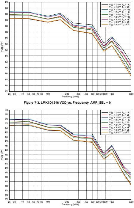
Figure 7-4. LMK1D1216 VOD vs. Frequency, AMP\_SEL = 1
