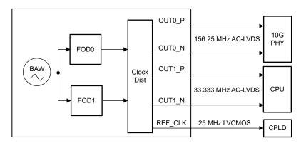
Figure 9-2. 10 Gb Ethernet Switch
