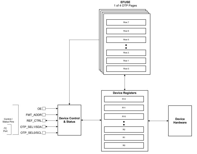
Figure 8-3. LMK3H0102 Interface and Control Blocks
