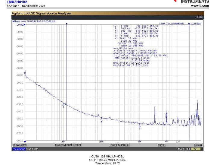
Figure 9-7. 125-MHz LP-HCSL on OUT0 with 156.25-MHz LP-HCSL on OUT1
