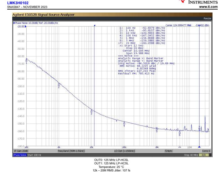
Figure 9-5. 125-MHz LP-HCSL Output, Measured on OUT0
