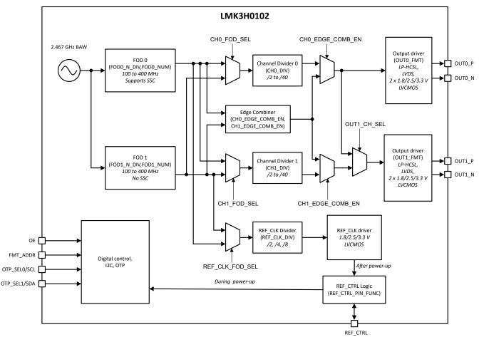
Figure 8-1. LMK3H0102 Functional Block Diagram
