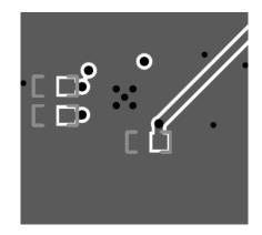
Figure 9-10. PCB Layout Example for LMK3H0102, Bottom Layer
