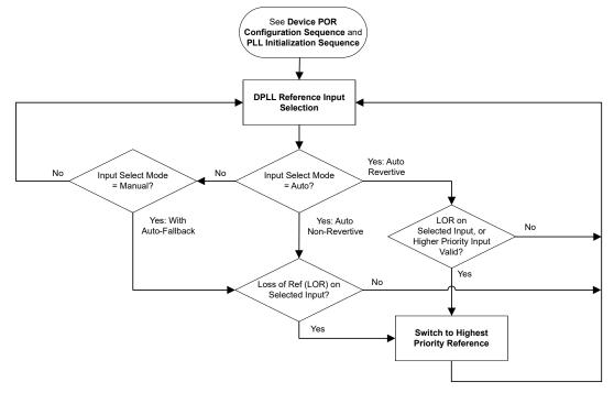
Figure 8-14. DPLL Reference Input Selection Flowchart
