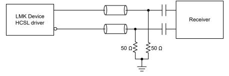
Figure 8-28. AC-Coupled HCSL Output Termination
