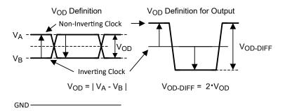
Figure 7-2. Two Different Definitions for Differential Output Signals
