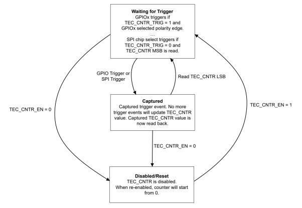
Figure 8-31. State Diagram of TEC
