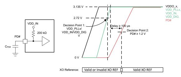
Figure 9-2. Recommendation for Power Up From Split-Supply Rails
