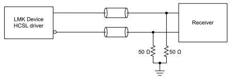
Figure 8-27. DC-Coupled HCSL Output Termination
