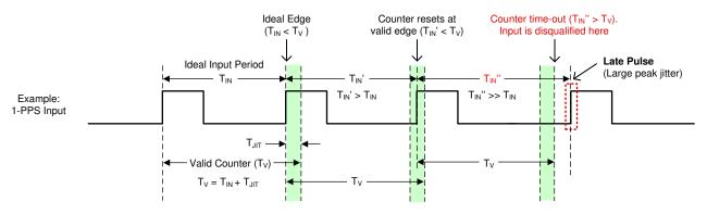
Figure 8-17. 1-PPS Input Window Detector Example
