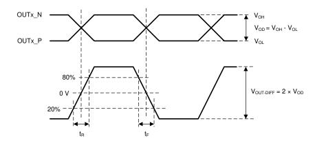
Figure 6-5. Differential Output Voltage and Rise/Fall Time
