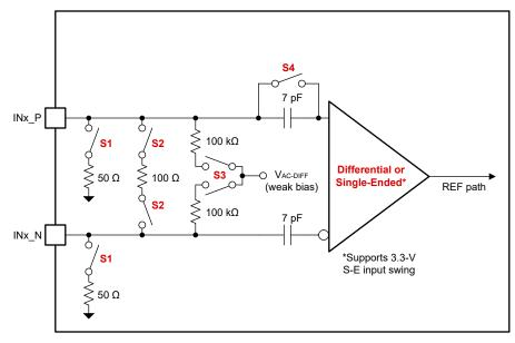
Figure 8-9. Reference Input Buffer
