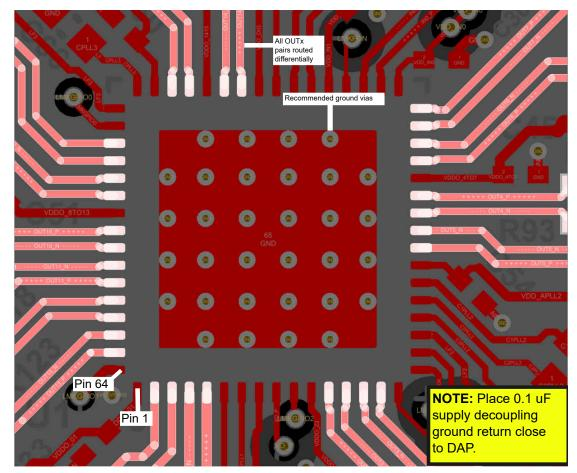
Figure 9-18. PCB Layout Example for LMK5B33216, Top Layer
