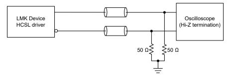
Figure 7-7. HCSL Output Time Domain Test Configuration
