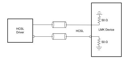
Figure 8-13. HCSL (Load Terminated) to Reference (INx)
