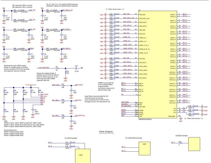
Figure 9-3. Reference Schematic Example
