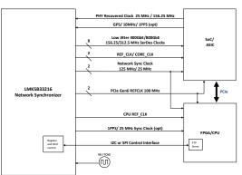
LMK5B33216 Typical System Block Diagram
