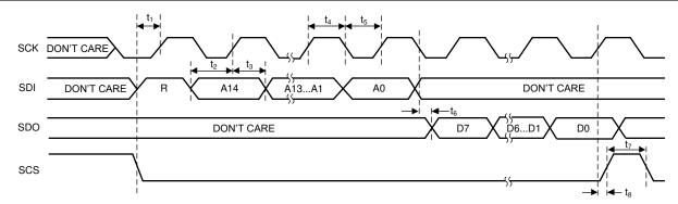
Figure 6-2. SPI 4-Wire Read Timing Diagram
