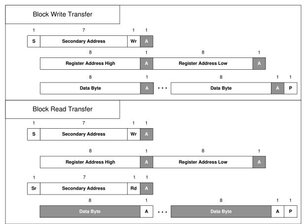
Figure 8-41. I<sup>2</sup>C Block Register Transfers
