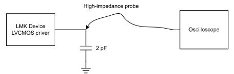
Figure 7-3. LVCMOS Output Time Domain Test Configuration
