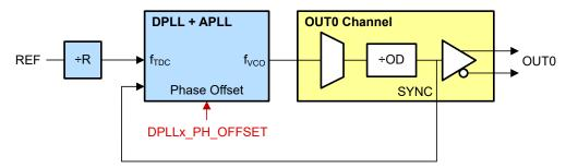
Figure 8-29. DPLL ZDM Synchronization Between Reference Input and OUT0
