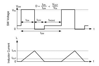
In auto mode, the low-side device is turned off once SW node current is near zero. As a result, once output current is less than half of what inductor ripple would be in CCM, the part operates in DCM which is equivalent to the statement that diode emulation is active.
