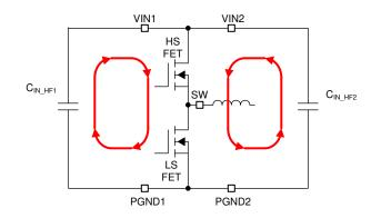
Figure 11-1. Input Current Loop
