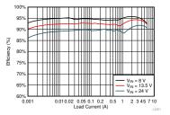
Efficiency: V<sub>OUT</sub> = 5 V, F<sub>SW</sub> = 2.1 MHz
