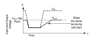
Whether output voltage falls due to high load or low input voltage, once the condition that causes output to fall below its set point is removed, the output climbs at the same speed as during start-up. Even though hiccup does not trigger due to dropout, it can in principle be triggered during recovery if output voltage is below 0.4 times the output set point for more than 128 clock cycles.
