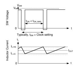
Figure 8-19. Current Limit Waveforms
