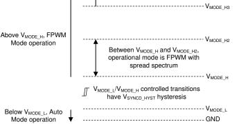
Figure 8-2. Level-Dependent Mode Selection Settings
