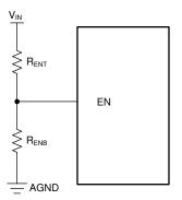
Figure 8-1. VIN/UVLO Using the EN pin
