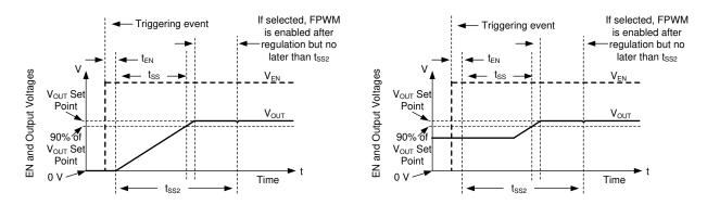
Soft start works with both output voltage starting from 0 V on the left curves, or if there is already voltage on the output, as shown on right. In either case, output voltage must reach within 10% of the desired value  $t_{SS}$  after soft start is initiated. During soft start, FPWM and hiccup are disabled. Both hiccup and FPWM are enabled once output reaches regulation or  $t_{SS2}$ , whichever happens first.
