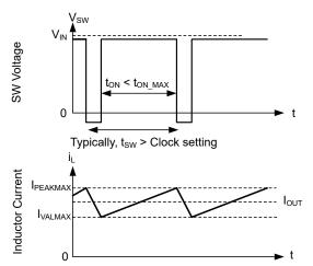
Figure 8-10. Current Limit Waveforms
