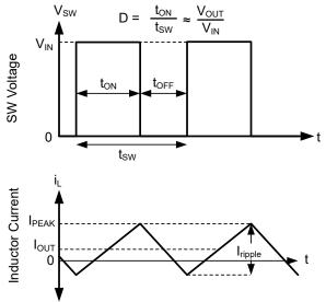
In FPWM mode, continuous conduction (CCM) is possible even if  $I_{OUT}$  is less than half of  $I_{ripple}$ .
