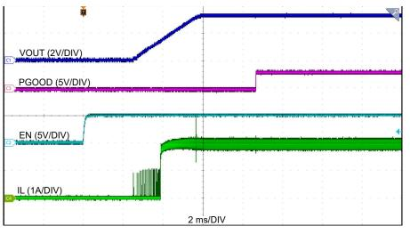
Figure 8-3. Enable Start-Up  $V_{IN}$  = 24 V,  $V_{OUT}$  = 3.3 V,  $I_{OUT}$  = 2 A
