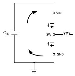
Figure 9-12. Current Loops with Fast Edges
