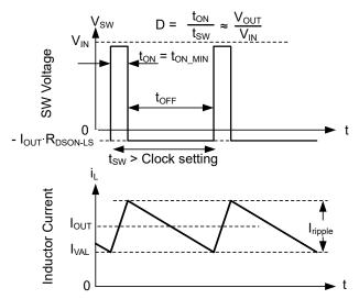
In valley control mode, minimum inductor current is regulated, not peak inductor current.
