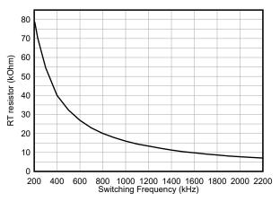
Figure 8-4. RT Values vs Frequency
