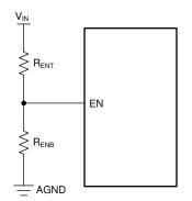
Figure 8-1. VIN UVLO Using the EN Pin
