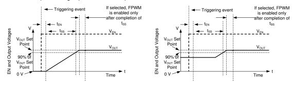
Figure 8-7. Soft Start with and Without Pre-bias Voltage
