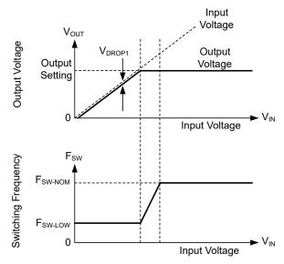
Output voltage and frequency versus input voltage: If there is little difference between input voltage and output voltage setting, the IC reduces frequency to maintain regulation. If input voltage is too low to provide the desired output voltage at F<sub>SW-LOW</sub> which is approximately 110-kHz, input voltage tracks output voltage.
