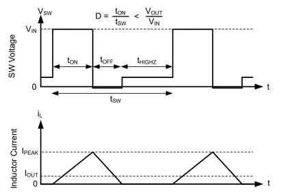
In auto mode, the low-side device is turned off after SW node current is near zero. As a result, after output current is less than half of what inductor ripple can be in CCM, the part operates in DCM, which is equivalent to the statement that diode emulation is active.
