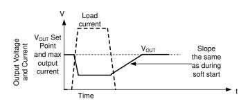
Figure 8-8. Recovery from Dropout
