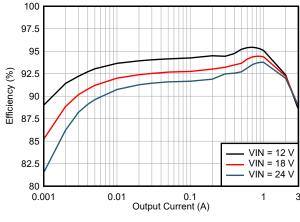
Efficiency: V<sub>OUT</sub> = 5 V (Fixed), 400 kHz
