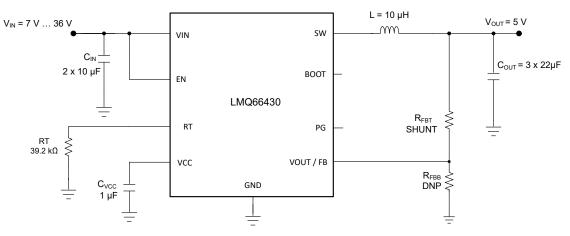
Figure 9-1. Application Circuit - 5 V (Fixed), 3 A, 400 kHz
