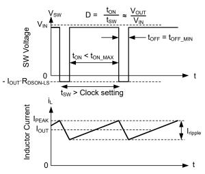
Switching waveforms while in dropout. Inductor current takes longer than a normal clock to reach the desired peak value. As a result, frequency drops. This frequency drop is limited by t<sub>ON-MAX</sub>.
