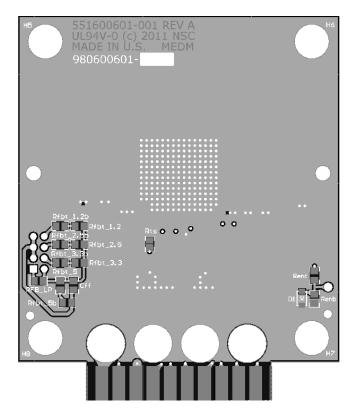
Figure 59. Bottom View of Evaluation PCB
