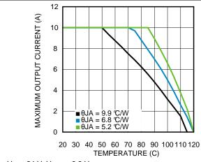
$V_{IN} = 24 \text{ V}, V_{OUT} = 3.3 \text{ V}$
