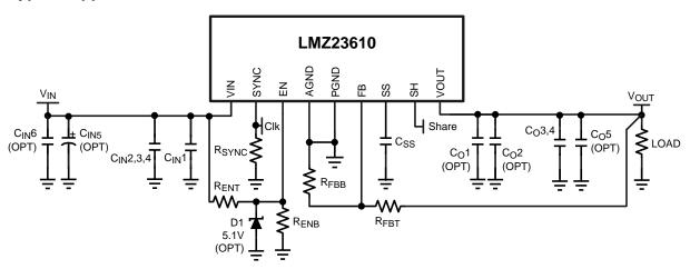
Figure 51. Typical Application Schematic Diagram
