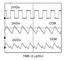
$V_{IN}$  = 12 V,  $V_{O}$  = 3.3 V,  $I_{O}$  = 3 A / 0.3 A
