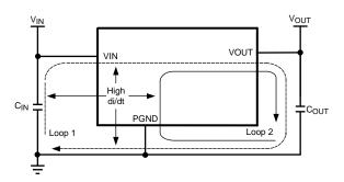
Figure 56. Critical Current Loops to Minimize
