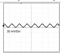
TIME (2 µs/Div) 12  $V_{IN}$ , 5  $V_{OUT}$  at Full Load, BW = 20 MHz
