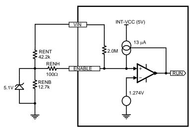
Figure 52. Enable Input Detail
