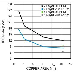
Figure 32. R<sub>J0A</sub> vs Copper Heat Sinking Area
