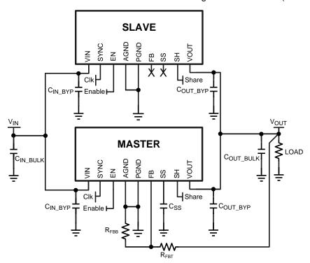
Figure 45. Current Sharing Example Schematic
