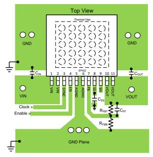
Figure 57. PCB Layout Guide
