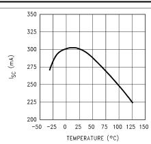
Figure 5-32. Instantaneous Short-Circuit Current versus Temperature (Legacy chip)
