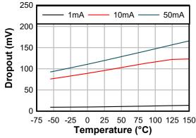
**Dropout Voltage versus Temperature (New Chip)**
