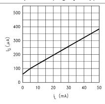
Figure 5-15. Ground Pin Current versus Load Current (Legacy Chip)
