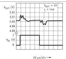
Figure 5-21. Line Transient Response (Legacy chip)
