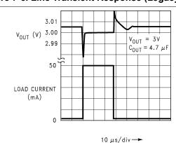
Figure 7-8. Load Transient Response (Legacy chip)
