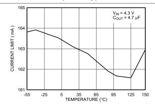
Figure 5-33. Short-Circuit Current versus Temperature (New Chip)
