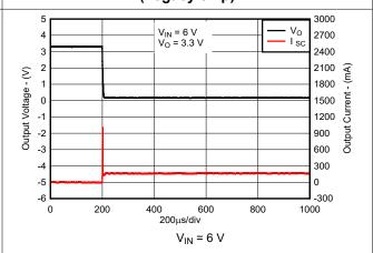
Figure 5-30. Short-Circuit Current versus Time (New Chip)
