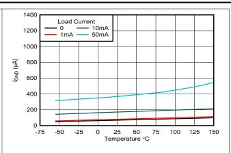
Figure 5-14. Ground Pin Current versus Temperature (New Chip)
