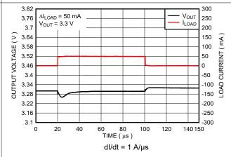
Figure 7-12. Load Transient Response (New Chip)
