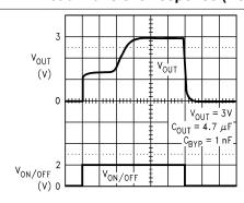
Figure 7-14. Turnon Waveform (Legacy chip)
