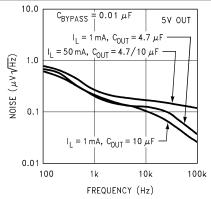
Figure 5-45. Output Noise Density (Legacy chip)
