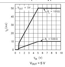
Figure 5-18. Input Current versus  $V_{IN}$  (Legacy Chip)
