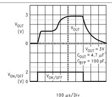
Figure 7-13. Turnon Waveform (Legacy chip)
