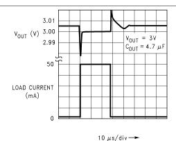
Figure 5-23. Load Transient Response (Legacy chip)
