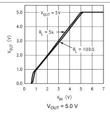
Figure 5-5. Output Voltage versus V<sub>IN</sub> (Legacy Chip)
