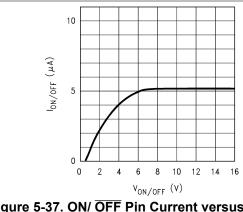
Figure 5-37. ON/ OFF Pin Current versus V<sub>ON/OFF</sub> (Legacy chip)
