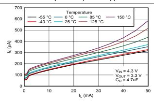
Figure 5-16. Ground Pin Current versus Load Current (New Chip)
