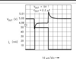
Figure 5-25. Load Transient Response (Legacy chip)
