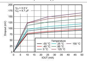
Figure 5-12. Dropout Voltage versus Load Current (New Chip)
