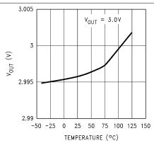
Figure 5-3. Output Voltage versus Temperature (Legacy Chip)
