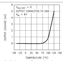
Figure 5-42. Input-to-Output Leakage versus Temperature (Legacy chip)
