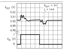
Figure 7-6. Line Transient Response (Legacy chip)
