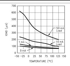
Figure 5-13. Ground Pin Current versus Temperature (Legacy Chip)
