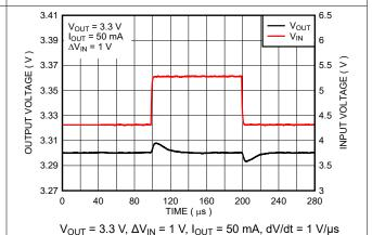
Figure 5-22. Line Transient Response (New Chip)
