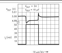
Figure 5-26. Load Transient Response (Legacy chip)
