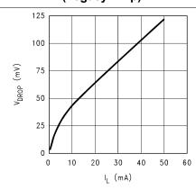
Figure 5-11. Dropout Voltage versus Load Current (Legacy Chip)
