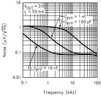
Figure 5-47. Output Noise Density (Legacy chip)
