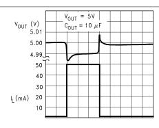
Figure 7-11. Load Transient Response (Legacy chip)
