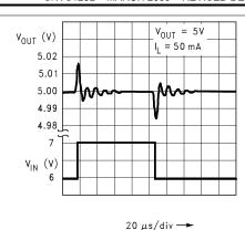
Figure 5-20. Line Transient Response (Legacy chip)
