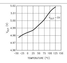
Figure 5-1. Output Voltage versus Temperature (Legacy Chip)
