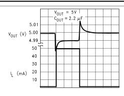
Figure 7-10. Load Transient Response (Legacy chip)
