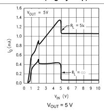
Figure 5-17. Input Current versus  $V_{\text{IN}}$  (Legacy Chip)
