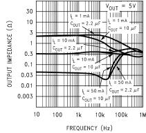
Figure 5-35. Output Impedance versus Frequency (Legacy chip)
