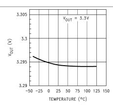
Figure 5-2. Output Voltage versus Temperature (Legacy Chip)
