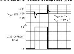
Figure 5-24. Load Transient Response (Legacy chip)
