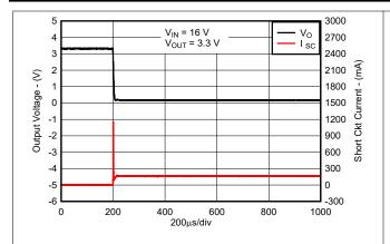
Figure 5-31. Short-Circuit Current versus Time (New Chip)
