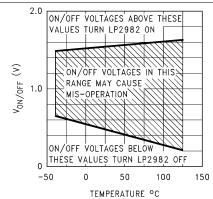
Figure 5-40. ON/ OFF Threshold versus Temperature (Legacy chip)
