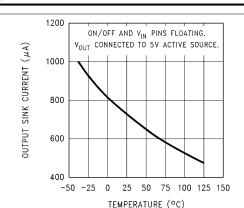
Figure 5-43. Output Reverse Leakage versus Temperature (Legacy chip)
