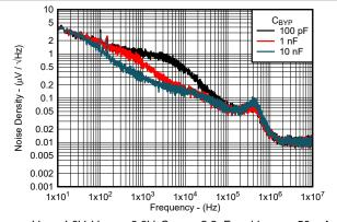
$V_{IN}$  = 4.3V,  $V_{OUT}$  = 3.3V,  $C_{OUT}$  = 2.2 $\mu F$  and  $I_{LOAD}$  = 50 mA
