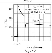
Figure 5-28. Short-Circuit Current versus Time (Legacy chip)
