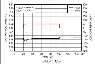
Figure 5-27. Load Transient Response (New Chip)
