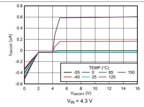
Figure 5-39. ON/OFF Pin Current versus V<sub>ON/OFF</sub> (New Chip)
