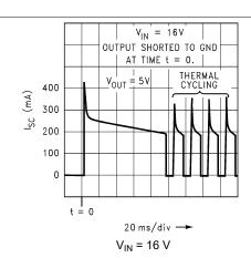
Figure 5-29. Short-Circuit Current versus Time (Legacy chip)
