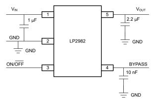
ON/ OFF input must be actively terminated. Tie to V<sub>IN</sub> if this function is not to be used. Minimum output capacitance is shown to insure stability over full load current range. More capacitance provides better dynamic performance and additional stability margin (see Section 7.1.1).
