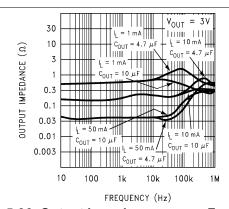
Figure 5-36. Output Impedance versus Frequency (Legacy chip)
