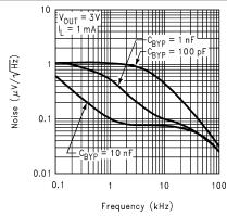
Figure 5-46. Output Noise Density (Legacy chip)
