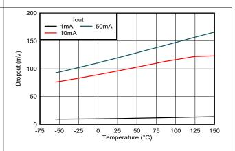
Figure 5-10. Dropout Voltage versus Temperature (New Chip)
