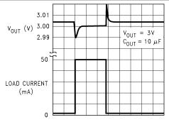
Figure 7-9. Load Transient Response (Legacy chip)
