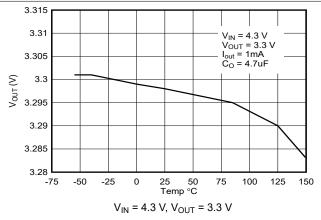
Figure 5-4. Output Voltage versus Temperature (New Chip)
