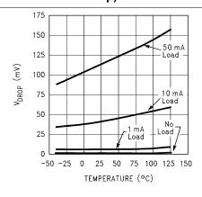
Figure 5-9. Dropout Voltage versus Temperature (Legacy Chip)
