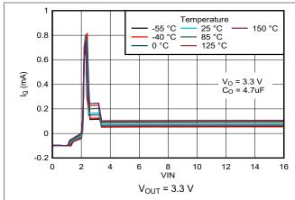
Figure 5-19. Input Current versus Input Voltage (New Chip)
