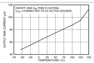
Figure 5-44. Output Reverse Leakage versus Temperature (New chip)
