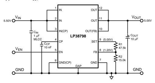
Figure 40. Typical Application, V<sub>OUT</sub> = 5 V
