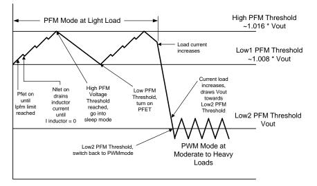
Figure 31. Operation in PFM Mode and Transfer to PWM Mode
