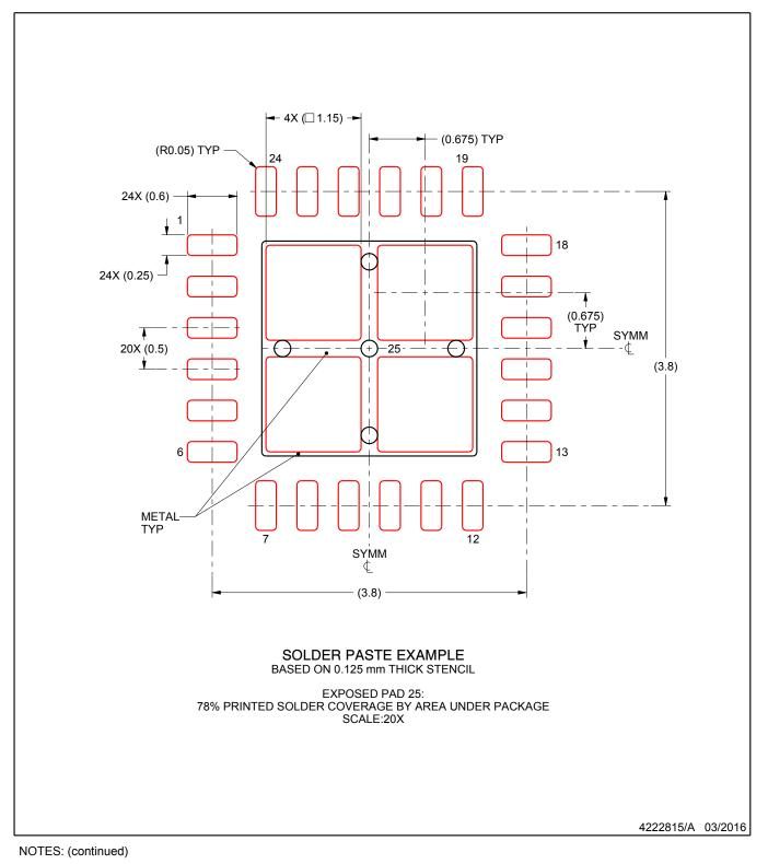
5. Laser cutting apertures with trapezoidal walls and rounded corners may offer better paste release. IPC-7525 may have alternate design recommendations.
