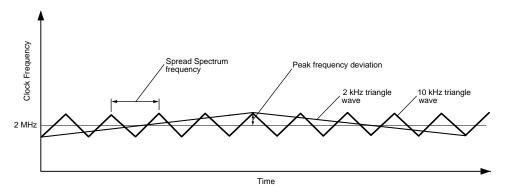
Figure 44. Spread Spectrum Modulation Frequency
