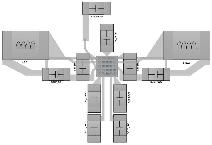
Figure 49. LP3907-Q1 DSBGA Layout Example
