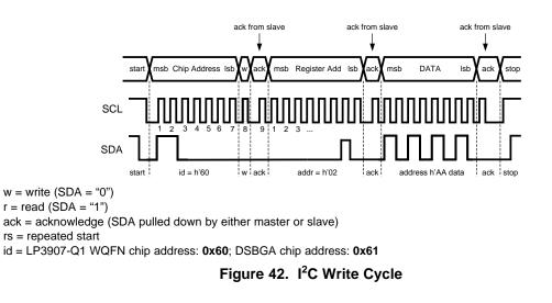
When a READ function is to be accomplished, a WRITE function must precede the READ function, as shown in the Read Cycle waveform.
