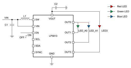
Figure 9-9. Mix drive, 1 scan (led\_mode = 5h, scan\_order\_0 = 0h, mix\_sel\_led = 8h)
