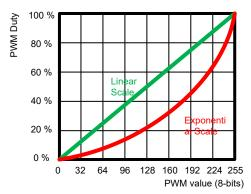
Figure 9-15. Linear and Exponential PWM Dimming Curves
