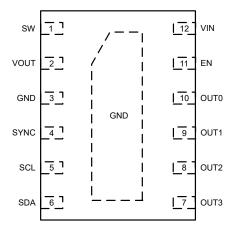
Figure 6-2. LP5813 DRR Package 12-Pin WSON Top View
