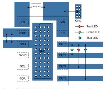
Figure 10-22. LP5813 WSON Package Layout Example
