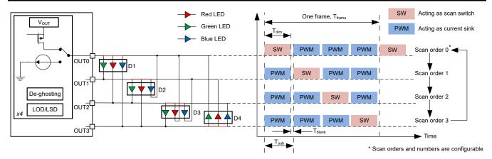
Figure 9-3. Time-cross-multiplexing (TCM) Scheme
