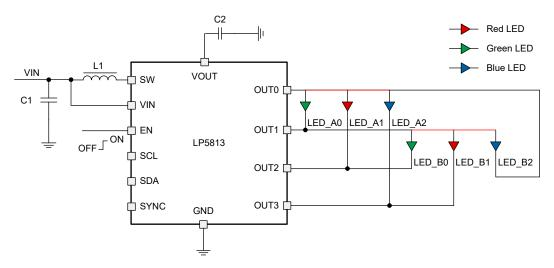
Figure 9-6. TCM Drive Mode, 2 Scans (led\_mode = 2h, scan\_order\_0 = 0h, scan\_order\_1 = 1h)
