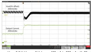
$V_{IN}$  = 3.6 V,  $V_{OUT}$  = 5 V,  $I_{OUT}$  = 400 mA to 800 mA with 20- $\mu$ s slew rate
