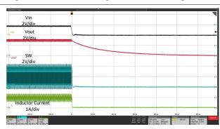
$V_{IN}$  = 2.0 V,  $V_{OUT}$  = 3.3 V, 6.6- $\Omega$  resistance load
