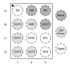
Figure 6-1. LP5813 YBH Package 12-Pin DSBGA Top View
