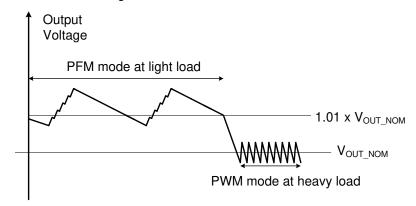
Figure 9-2. Output Voltage in PWM Mode and PFM
