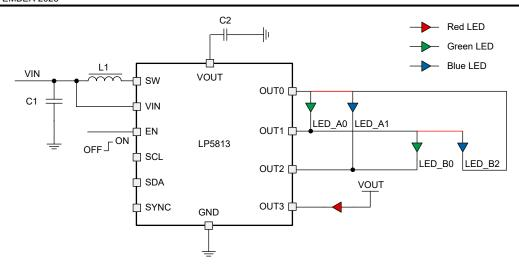
Figure 9-10. Mix drive mode, 2 scans (led\_mode = 6h, scan\_order\_0 = 0h, scan\_order\_1 = 1h, mix\_sel\_led = 8h)
