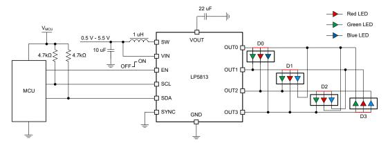
Figure 10-1. Typical Application - LP5813 Driving RGB LEDs
