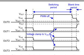
Figure 9-12. Ghosting elimination waveform when clamp\_sel = 1
