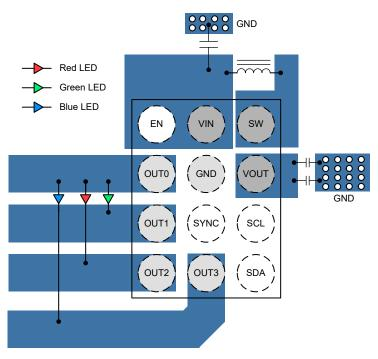
Figure 10-21. LP5813 DSBGA Package Layout Example
