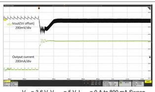
$V_{IN}$  = 3.6 V,  $V_{OUT}$  = 5 V,  $I_{OUT}$  = 0 A to 800 mA Sweep
