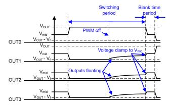
Figure 9-13. Ghosting elimination waveform when clamp\_sel = 0
