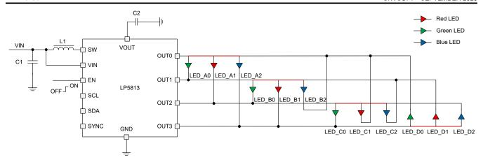
Figure 9-8. TCM Drive Mode, 4 Scans (led\_mode = 4h scan\_order\_0 = 0h, scan\_order\_1 = 1h, scan\_order\_2 = 2h, scan\_order\_3 = 3h)
