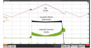
$V_{IN}$  = 0 V to 3 V Sweep,  $V_{OUT}$  = 3 V, 6.6- $\Omega$  resistance load
