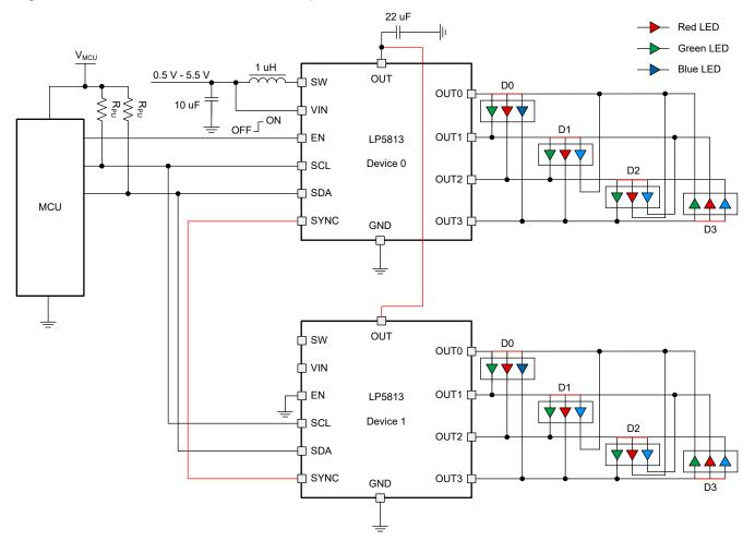
Figure 10-3. Typical Application - Dual LP5813 Application Example
