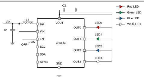
Figure 9-4. Direct Drive Mode (led\_mode = 0h)
