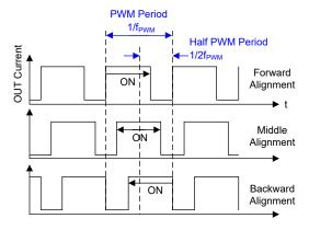
Figure 9-14. PWM Alignment Scheme
