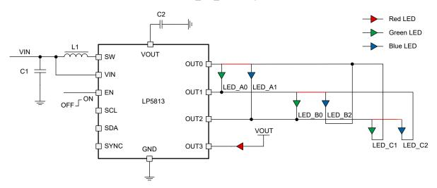
Figure 9-11. Mix drive mode, 3 scans (led\_mode = 7h, scan\_order\_0 = 0h, scan\_order\_1 = 1h, scan\_order\_2 = 2h, mix\_sel\_led = 8h)
