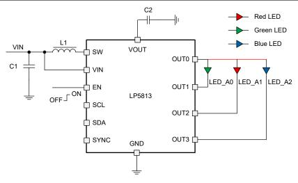
Figure 9-5. TCM Drive Mode, 1 Scan, (led\_mode = 1h, scan\_order\_0 = 0h)
