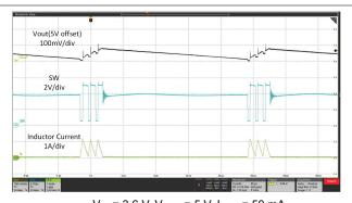
$V_{IN} = 3.6 \text{ V}, V_{OUT} = 5 \text{ V}, I_{OUT} = 50 \text{ mA}$
