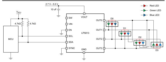
Figure 10-2. Typical Application - LP5813 Bypassing the Boost Converter
