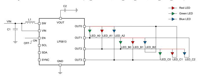
Figure 9-7. TCM Drive Mode, 3 Scans (led\_mode = 3h, scan\_order\_0 = 0h, scan\_order\_1 = 1h, scan\_order\_2 = 2h)
