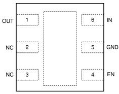
Figure 5-3. DRV Package, 6-Pin WSON With Thermal Pad, Top View
