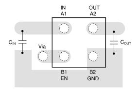
Figure 10-1. LP5910 Typical DSBGA Layout
