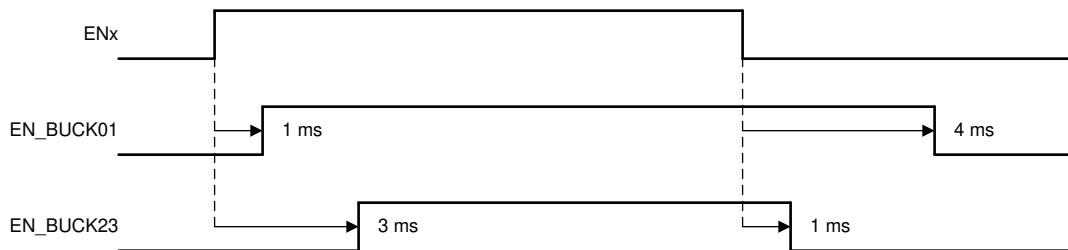
Figure 16. Typical Start-Up and Shutdown Sequencing
